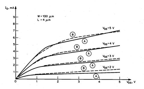
Figure 4.9. Drain current versus drain voltage characteristics of an n-channel MOSFET calculated with the LEVEL 2 model (A) and the LEVEL 3 model (B) (Copyright © 1988 by McGraw-Hill, Inc.).
