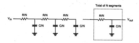
Figure 6.24. Distributed RC ladder network model consisting of N equal segments.
