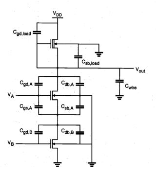
Figure 7.9. Parasitic device capacitances in the NAND2 gate.
