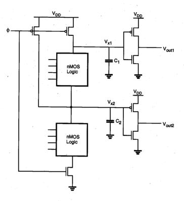
Figure 9.34. Precharging of internal nodes to prevent charge sharing also allows implementation of multiple-output domino CMOS structures.
