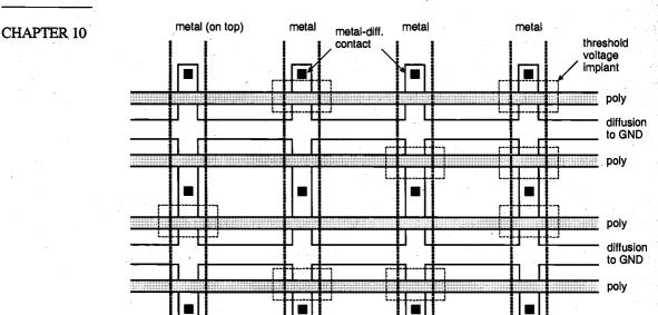
**Figure 10.7.** Layout of the 4-bit x 4-bit NOR ROM array example shown in Fig. 10.3. The threshold voltages of "1"-bit transistors are raised above  $V_{DD}$  through implant.
