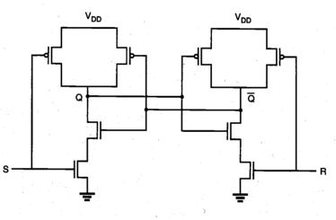
Figure 8.11. CMOS SR latch circuit based on NAND2 gates.
