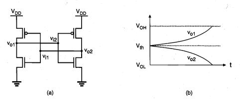
*Figure 8.3.* (a) Circuit diagram of a CMOS bistable element. (b) One possibility for the expected time-domain behavior of the output voltages, if the circuit is initially set at its unstable operating point.
