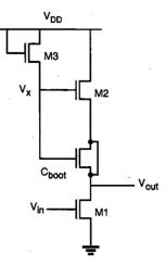
Figure 9.13. Realization of the bootstrapping capacitor with a dummy MOS device.
