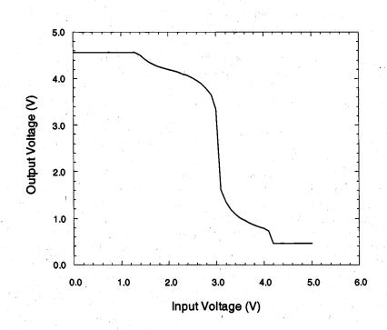
Figure 12.21. Typical voltage transfer characteristic of the BiCMOS inverter circuit.
