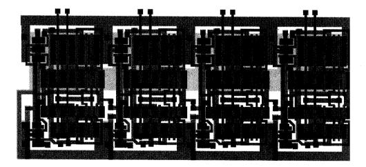
PLATE 10:(Top)Layout of a CMOS full adder (FA) circuit.<br/>(Bottom)(Bottom)Layout of a 4-bit ripple-carry adder, consisting of four FA cells.
