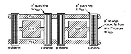
Figure 13.32. I/O cell layout with latch-up guidelines.
