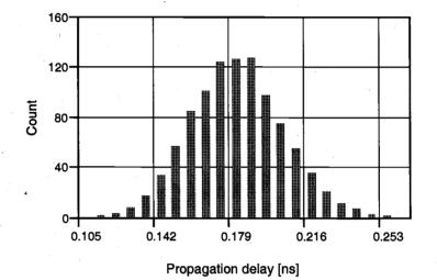
**Figure 15.6.** Histogram showing variation of  $\tau_P$  with  $V_{T,p}$ ,  $V_{T,p}$ , and  $t_{ox}$ .
