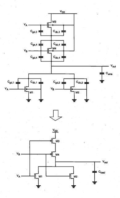
Figure 7.12. Parasitic device capacitances of the CMOS NOR2 circuit and the simplified equivalent with the lumped output load capacitance.
