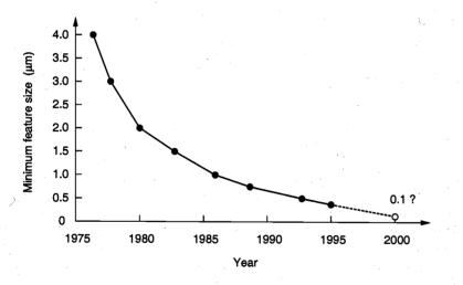
Figure 1.2. Evolution of minimum feature size in integrated circuits over time.
