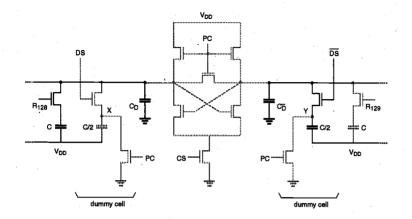
Figure 10.47. Two complementary column voltages are determined through charge sharing, on the one side between the selected storage cell and the half-column capacitance, on the other side between the dummy cell and the other half-column capacitance.
