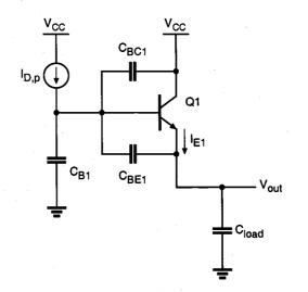
Figure 12.26. Equivalent circuit used for the pull-up delay analysis.
