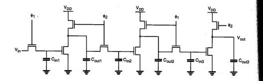
Figure 9.19. Enhancement-load dynamic shift register (ratioed logic).
