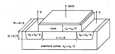
Figure 3.24. Scaling of a typical MOSFET by a scaling factor of S.
