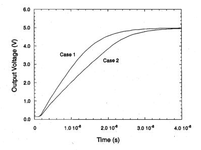
The simulated transient response of the NAND2 gate for both cases is plotted against time above. The time delay difference between the two cases is clearly visible. In fact, the propagation delay time in Case 2 is about 30% larger than that in Case 1, which proves that the input switching order has a significant influence on speed.
