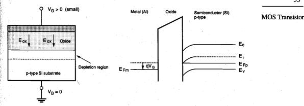
The cross-sectional view and the energy band diagram of the MOS structure Figure 3.6. operating in depletion mode, under small gate bias.
