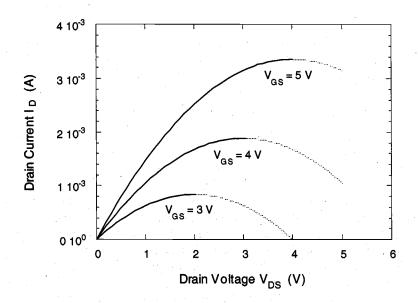
The drain current-drain voltage curves shown above reach their peak value for  $V_{DS} = V_{CS} - V_{T0}$ . Beyond this maximum, each curve exhibits a *negative* differential conductance, which is not observed in actual MOSFET current-voltage measurements (section shown by the dashed lines). We must remember now that the drain current equation (3.32) has been derived under the following voltage assumptions,
