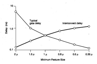
Figure 6.13. Interconnect delay dominates gate delay in submicron CMOS technologies.
