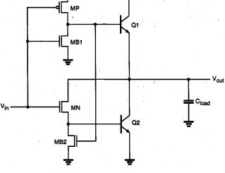
Figure 12.20. Conventional BiCMOS inverter circuit with active base pull-down.
