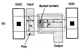
Figure 5.15. Sample layout of depletion-load inverter circuits (a) with output contact on diffusion and (b) with buried contact.
