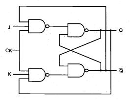
Figure 8.20. All-NAND implementation of the clocked JK latch circuit.
