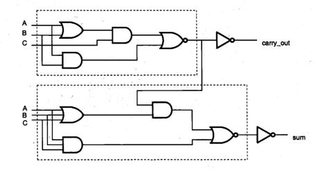
Figure 7.27. Gate-level schematic of the one-bit full-adder circuit.
