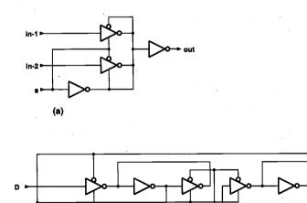
Figure 14.9. Regular design of (a) 2-1 MUX and (b) DFF, using inverters and tri-state buffers as basic building blocks.
