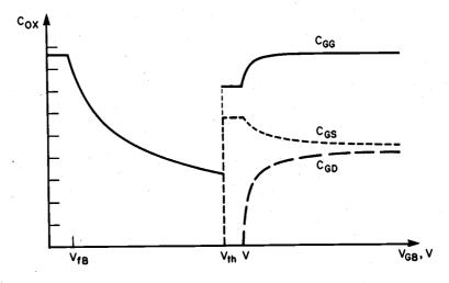
Figure 4.8. Oxide capacitances as functions of the gate-to-substrate voltage, according to Ward's capacitance model (Copyright © 1988 by McGraw-Hill, Inc.).
