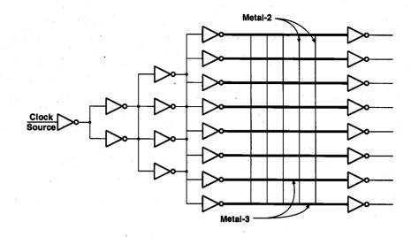
Figure 13.26. Genaral structure of the clock distribution network used in DEC Alpha microprocessor chips.
