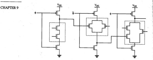
Figure 9.38. NORA CMOS logic circuit example.
