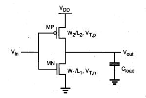
Figure 15.4. A CMOS inverter circuit.
