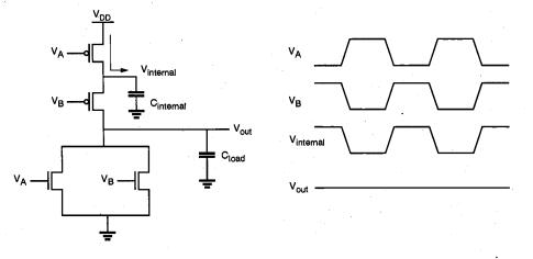
*Figure 11.3.* Switching of the internal node in a two-input NOR gate results in dynamic power dissipation even if the output node voltage remains unchanged.
