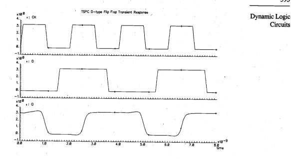
Figure 9.44. Simulation results showing the operation of the TSPC-based DFF circuit, with a clock frequency of 500 MHz.
