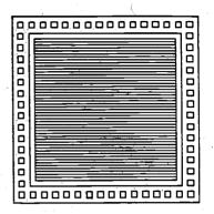
flexibility in channel definition (position & width) over-the-cell routing higher packing density RAM-compatible supports variable-height cells & macrocells
