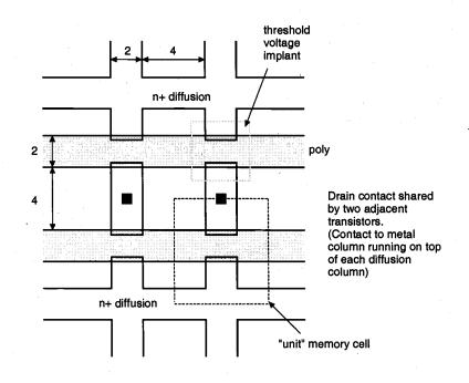
Figure 10.16. Simplified mask layout of the implant-mask programmable NOR ROM array considered in the example. All dimensions are in micrometers ( $W = 2 \ \mu m$ ,  $L = 1.5 \ \mu m$ ).
