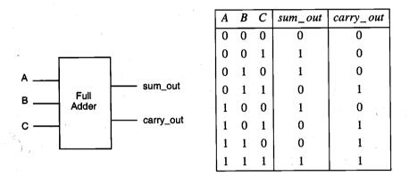
The sum\_out and carry\_out signals can be found as the following two combinational Boolean functions of the three input variables, A, B and C.
