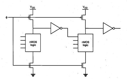
Figure 9.29. Cascaded domino CMOS logic gates.
