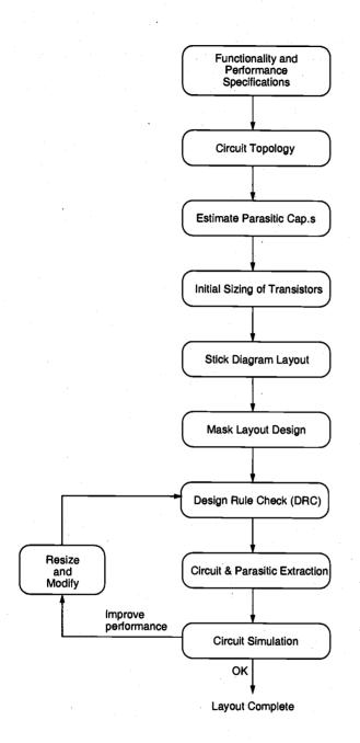
Figure 2.13. Typical design flow for the production of a mask layout.
