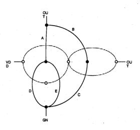
*Figure 7.18.* Construction of the dual pull-up graph from the pull-down graph, using the dual-graph concept.
