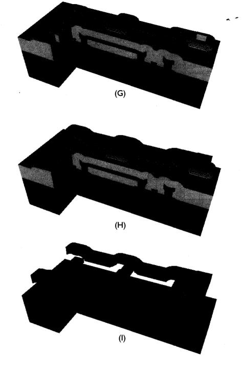
**PLATE 5:** Cross-sectional view showing the fabrication steps for a CMOS inverter (continued):
