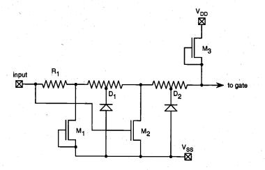
Figure 13.4. Protection network with thick-oxide transistor.
