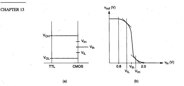
Figure 13.8. (a) TTL to CMOS level shifting and (b) the corresponding voltage transfer characteristic curve.
