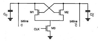
Figure 10.33. Cross-coupled nMOS sense amplifier circuit.
