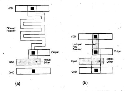
Figure 5.10. Sample layout of resistive-load inverter circuits with (a) diffused resistor and (b) undoped polysilicon resistor.
