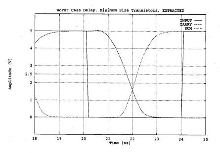
*Figure 1.12.* Simulated output waveforms of the full adder circuit with minimum transistor dimensions, showing the signal propagation delay during one of the worst-case transitions.
