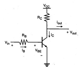
Figure 12.12. The resistive-load BJT inverter circuit.
