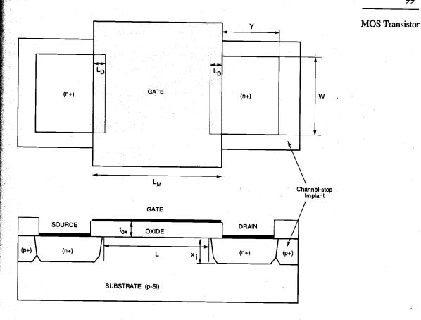
Figure 3.29. Cross-sectional view and top view (mask view) of a typical n-channel MOSFET.
