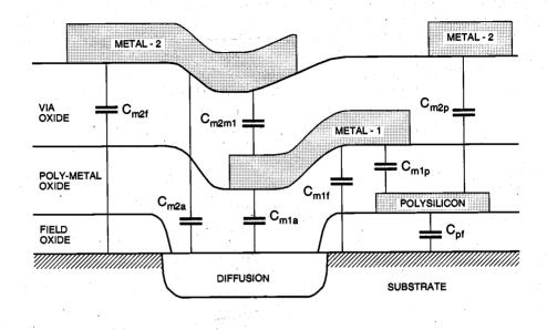
Figure 6.22. Cross-sectional view of a double-metal CMOS structure, showing capacitances between various layers.
