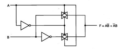
Figure 7.38. Eight-transistor CMOS TG implementation of the XOR function.
