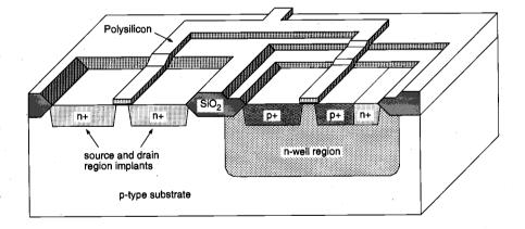
**Figure 2.8.** Using a set of two masks, the n+ and p+ regions are implanted into the substrate and into the n-well, respectively. Also, the ohmic contacts to the substrate and to the n-well are implanted in this process step. After *Atlas of IC Technologies*, by W. Maly [1].
