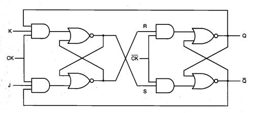
Figure 8.25. NOR-based realization of the JK master-slave flip-flop.
