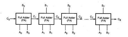
Figure 1.15. Block diagram of a carry ripple adder chain consisting of full adders.
