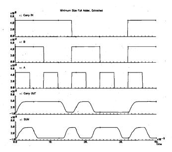
Figure 7.31. Simulated input and output waveforms of the CMOS full-adder circuit.
