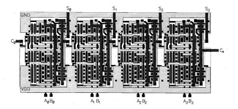
Figure 1.16. Mask layout of the 8-bit carry ripple adder array.
