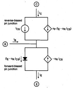
*Figure 12.8.* The Ebers-Moll equivalent circuit diagram of the npn BJT operating in the forward active mode.
