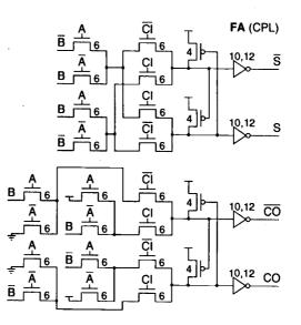
Figure 7.44. Circuit diagram of a CPL full adder.
