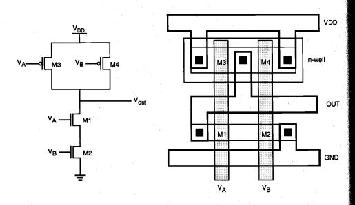
Figure 7.15. Sample layout of the CMOS NAND2 gate.
