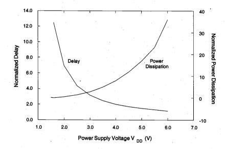
Figure 11.9. Normalized propagation delay and average switching power dissipation of a CMOS inverter, as a function of the power supply voltage  $V_{pp}$ .
