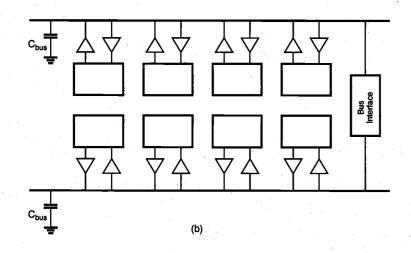
*Figure 11.25.* (a) Using a single global bus structure for connecting a large number of modules on chip results in large bus capacitance and large dynamic power dissipation. (b) Using smaller local buses reduces the amount of switched capacitance, at the expense of additional chip area.
