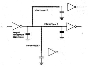
Figure 6.11. An inverter driving three other inverters over interconnection lines.
