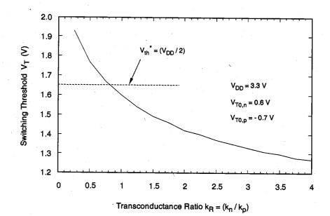
Figure 5.22. Variation of the inversion threshold voltage as a function of  $k_{\rm p}$ .
