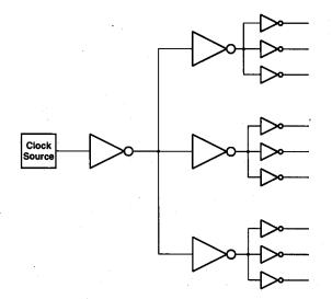
Figure 13.25. Three-level buffered clock distribution network.
