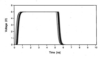
Figure 15.2. Process-related variation in output waveform of a 4-bit adder.
