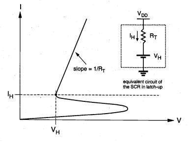
Figure 13.28. Current-voltage characteristics of a typical SCR.
