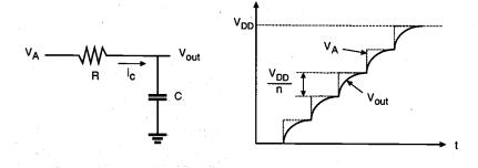
Figure 11.31. Equivalent circuit, and the input and output voltage waveforms of the CMOS inverter circuit shown in Fig. 11.30 (stepwise charge-up case).
