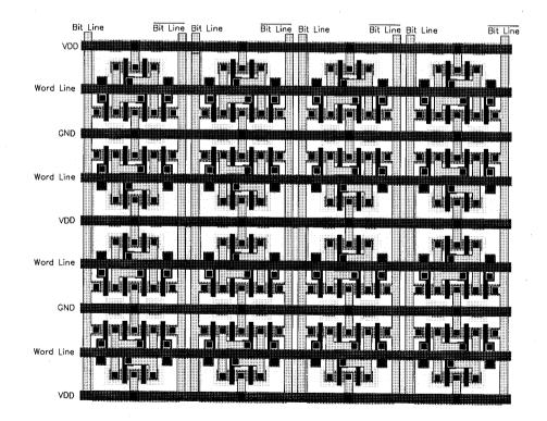
*Figure 10.25. (continued)* (b) Layout of the CMOS SRAM cell. (c) Layout of a 4-bit x 4-bit SRAM array, consisting of 16 CMOS SRAM cells.
