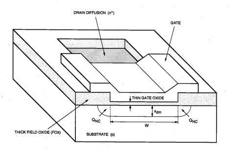
**Figure 3.26.** Cross-sectional view (across the channel) of a narrow-channel MOSFET. Note that  $Q_{NC}$  indicates the extra depletion charge due to narrow-channel effects.
