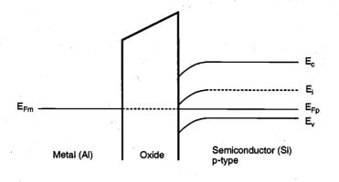
Figure 3.4. Energy band diagram of the combined MOS system.
