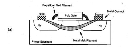
Figure 13.5. (a) Typical ESD failure modes.
