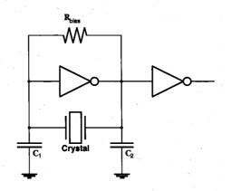
Figure 13.20. Circuit diagram of a Pierce crystal oscillator circuit.
