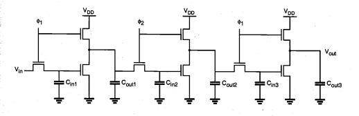
Figure 9.21. Enhancement-load dynamic shift register (ratioless logic).
