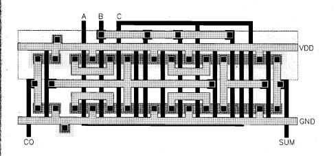
Figure 7.29. Mask layout of the CMOS full-adder circuit using minimum-size transistors.
