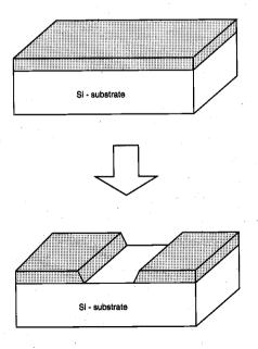
**Figure 2.3.** The result of a single lithographic patterning sequence on silicon dioxide, without showing the intermediate steps. Compare the unpatterned structure (top) and the patterned structure (bottom) with Fig. 2.2(b) and Fig. 2.2(g), respectively.
