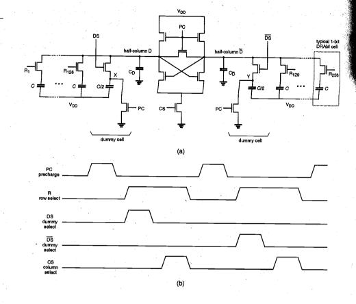
*Figure 10.45.* (a) Data read-restore circuit example for 256 1-T DRAM cells per column. (b) Typical control signal waveforms for two consecutive data read operations, performed on alternate sides (half-columns) of the array.
