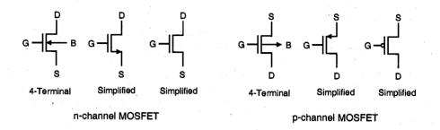
Figure 3.9. Circuit symbols for n-channel and p-channel enhancement-type MOSFETs.
