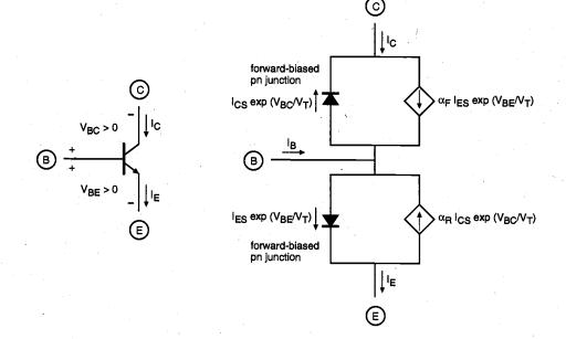
Figure 12.11. The Ebers-Moll equivalent circuit diagram of the npn BJT operating in saturation mode.
