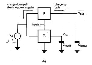
*Figure 11.28.* (a) The general circuit topology of a conventional CMOS logic gate. (b) The topology of an adiabatic logic gate implementing the same function. Note the difference in charge-up and charge-down paths for the output capacitance.
