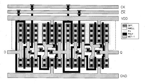
Figure 8.33. Layout of the CMOS DFF shown in Fig. 8.30.
