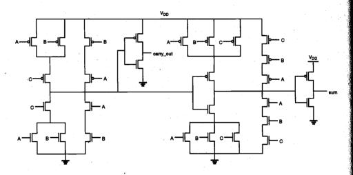
Figure 7.28. Transistor-level schematic of the one-bit full-adder circuit.
