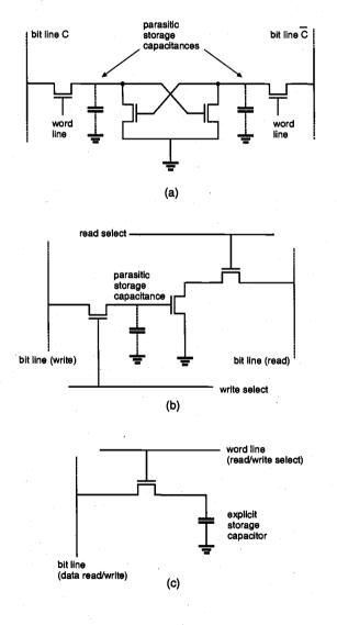
**Figure 10.36.** Various configurations of the dynamic RAM cell. (a) Four-transistor DRAM cell with two storage nodes. (b) Three-transistor DRAM cell with two bit lines and two word lines. (c) One-transistor DRAM cell with one bit line and one word line.
