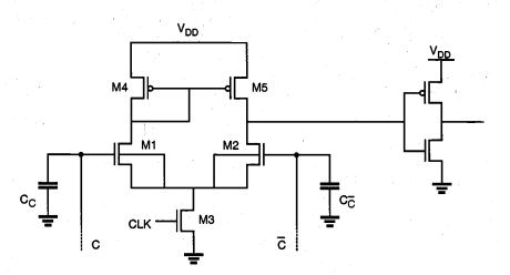
Figure 10.30. Differential current-mirror amplifier to speed up the memory read access time.
