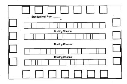
Figure 14.20. A simplified floorplan of standard-cell-based design.
