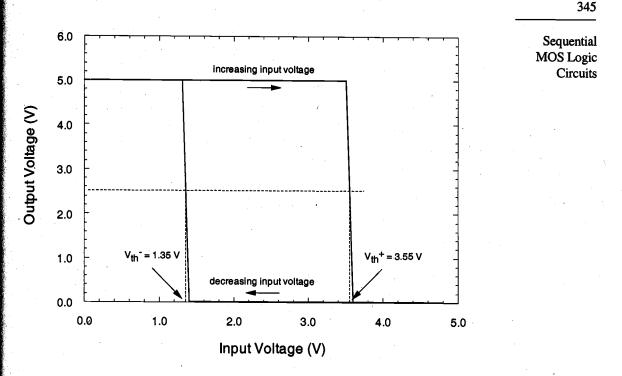
Figure 8.36. Simulated output voltage waveforms of the CMOS Schmitt trigger circuit, for increasing and for decreasing input voltage.
