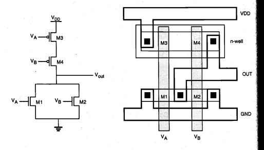
Figure 7.14. Sample layout of the CMOS NOR2 gate.
