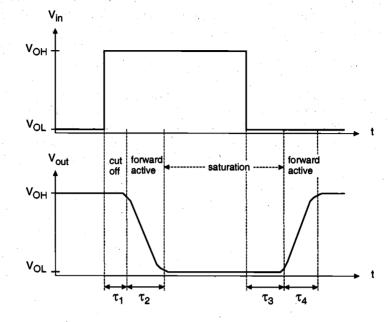
Figure 12.18. Typical input and output voltage waveforms of the BJT inverter during transient operation.
