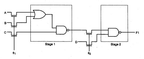
Figure 9.17. A two-stage synchronous complex logic circuit example.
