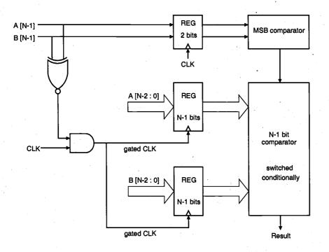
Figure 11.24. Block diagram of an N-bit number comparator with gated clock scheme.
