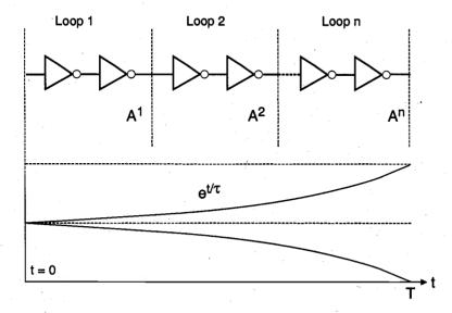
Figure 8.6. Propagation of a transient signal in the two-inverter loop during settling.
