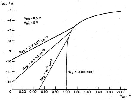
**Figure 4.7.** Variation of the drain current in the weak inversion region, as a function of the gate voltage and for different values of the parameter  $N_{FS}$ , in the LEVEL 2 model (Copyright © 1988 by McGraw-Hill, Inc.).
