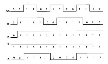
Figure 8.35. Timing diagram of the positive edge-triggered D flip-flop.
