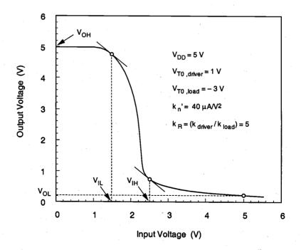
Figure 5.13. Typical VTC of a depletion-load inverter circuit.
