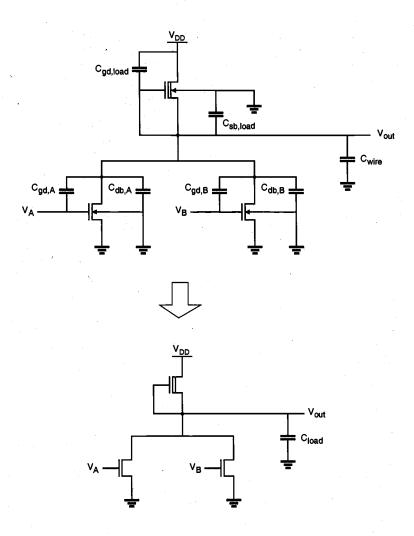
*Figure 7.5.* Parasitic device capacitances in the NOR2 gate and the lumped equivalent load capacitance. The gate-to-source capacitances of the driver transistors are included in the load of the previous stages driving the inputs A and B.
