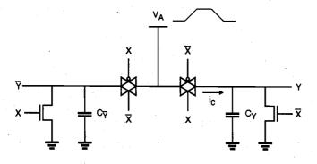
Figure 11.27. Adiabatic amplifier circuit which transfers the complementary input signals to its complementary outputs through CMOS transmission gates.
