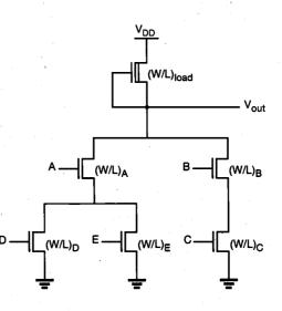
Figure 7.17. nMOS complex logic gate realizing the Boolean function given in (7.41).
