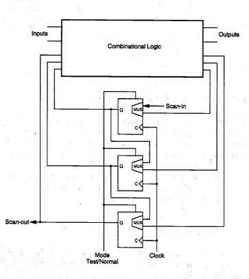
Figure 16.9. The general structure of scan-based design.
