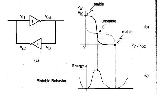
**Figure 8.2.** Static behavior of the two-inverter basic bistable element: (a) Circuit schematic. (b) Intersecting voltage transfer curves of the two inverters, showing the three possible operating points. (c) Qualitative view of the potential energy levels corresponding to the three operating points.
