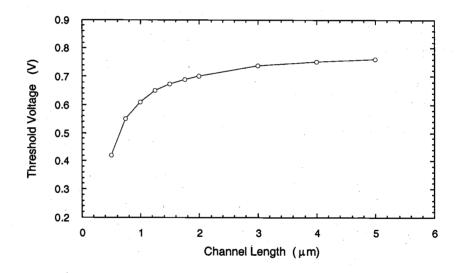
Since the conventional threshold voltage expression (3.23) is not capable of accounting for this drastic reduction of  $V_{T0}$  at smaller channel lengths, its application for short-channel MOSFETs must be carefully restricted.
