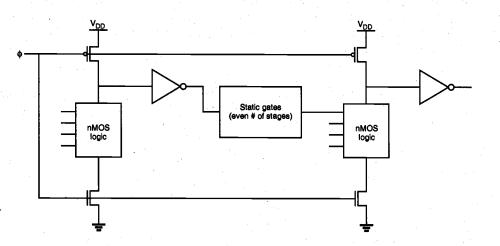
Figure 9.31. Cascading domino CMOS logic gates with static CMOS logic gates.
