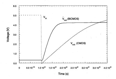
**Figure 12.22.** Simulated output voltage waveforms of a conventional CMOS inverter and a BiCMOS inverter, both driving a capacitive load of 5 pF. Note that both circuits also occupy approximately the same amount of silicon area.
