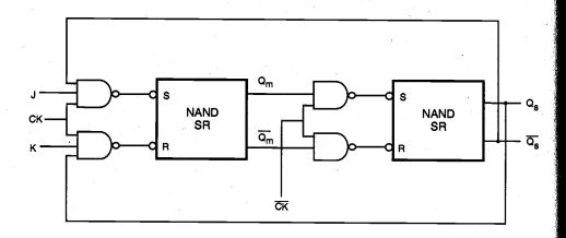
Figure 8.23. Master-slave flip-flop consisting of NAND-based JK latches.
