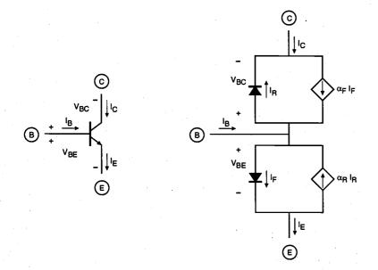
Figure 12.7. The Ebers-Moll equivalent circuit diagram of the npn BJT.
