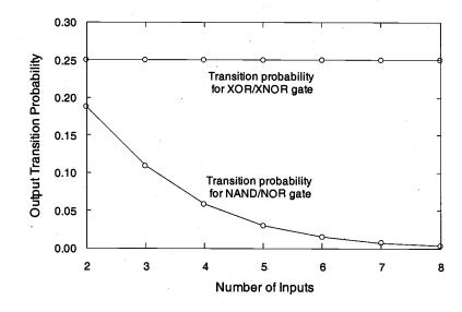
*Figure 11.20.* Output transition probabilities of different logic gates, as a function of the number of inputs. Note that the transition probability of the XOR gate is independent of the number or inputs.
