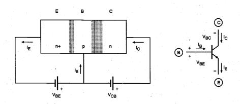
Figure 12.6. The simplified view of the bipolar junction transistor (BJT) biased in the forward active mode with  $V_{BE}$  and  $V_{CB}$ , and the corresponding circuit symbol. Note that the depletion regions at both pn junctions are also highlighted.
