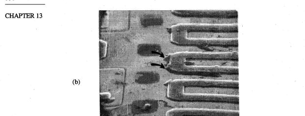
Figure 13.5. (b) SEM photograph of a failed nMOS transistor (from Reference 7).
