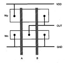
Figure 7.16. Stick-diagram layout of the CMOS NOR2 gate.
