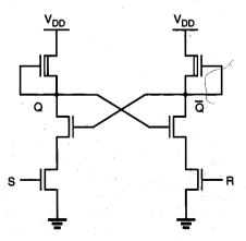
Figure 8.13. Depletion-load nMOS NAND-based SR latch circuit.
