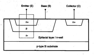
Figure 12.5. Cross-section of an npn-type bipolar junction transistor (BJT).
