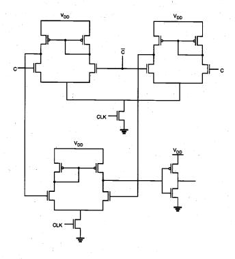
Figure 10.31. Two-stage differential current-mirror sense amplifier circuit.
