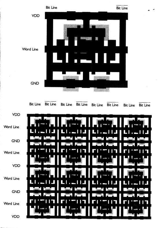
PLATE 9: (Top) Layout of a CMOS SRAM cell. (Bottom) Layout of a 4x4 SRAM array, consisting of 16 cells.
