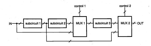
Figure 16.5. Partition-and-mux method for large circuits.
