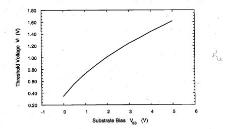
Variation of the threshold voltage as a function of the source-to-substrate voltage.
