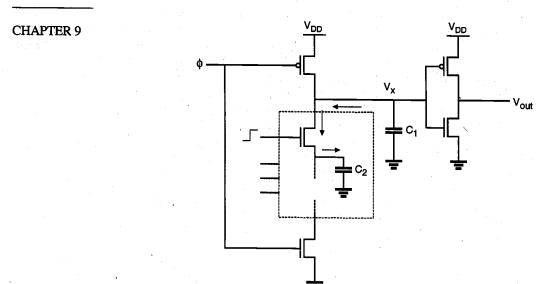
**Figure 9.32.** Charge sharing between the output capacitance  $C_1$  and an intermediate node capacitance  $C_2$  during the evaluation cycle may reduce the output voltage level.
