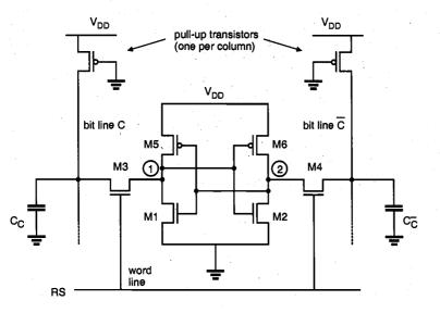
Figure 10.24. Circuit topology of the CMOS SRAM cell.
