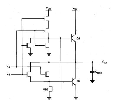
Figure 12.30. Circuit diagram of the BiCMOS NOR2 gate.
