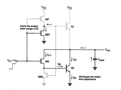
Figure 12.28. BiCMOS inverter during a transient output pull-down event. The active devices in the circuit are highlighted (darker).
