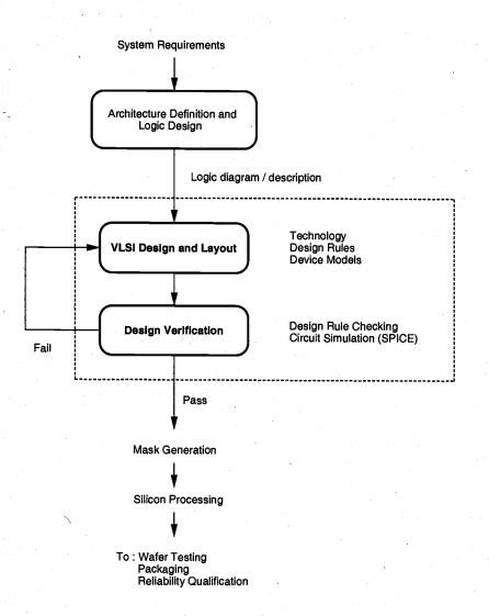
Figure 1.6. The flow of circuit design procedures.
