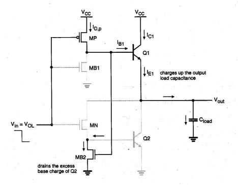
Figure 12.25. BiCMOS inverter during transient output pull-up event. The active devices in the circuit are highlighted (darker).
