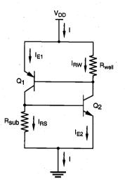
Figure 13.29. Equivalent circuit model for the SCR.
