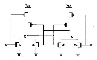
Figure 8.7. CMOS SR latch circuit based on NOR2 gates.
