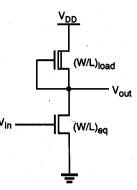
Figure 7.4. Equivalent inverter circuit corresponding to the *n*-input NOR gate.
