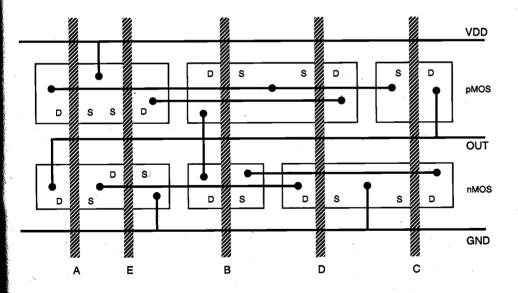
Figure 7.20. Stick-diagram layout of the complex CMOS logic gate, with an arbitrary ordering of the polysilicon gate columns.
