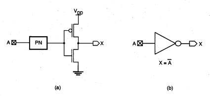
Figure 13.7. Inverting input circuit with (a) protection network, and (b) symbolic view.
