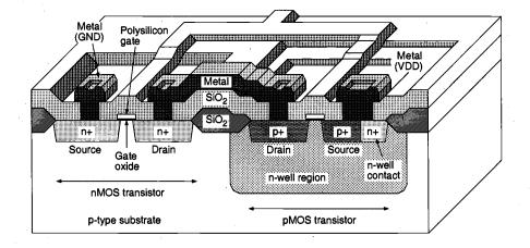
*Figure 2.11.* The composite layout and the resulting cross-sectional view of the chip, showing one nMOS and one pMOS transistor (in the n-well), and the polysilicon and metal interconnections. The final step is to deposit the passivation layer (for protection) over the chip, except over wire-bonding pad areas. After *Atlas of IC Technologies*, by W. Maly [1].
