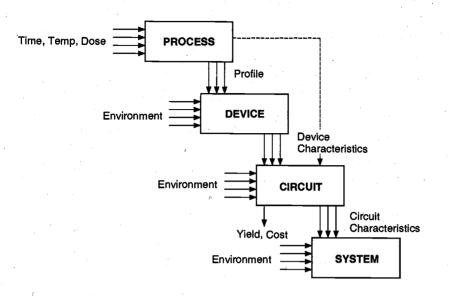
Figure 15.1. Relationship between process and device parameters and circuit and system performance.
