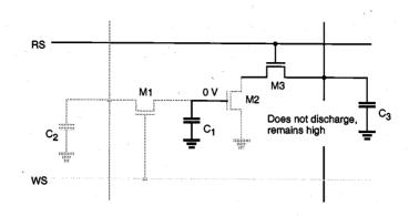
Figure 10.43. The column capacitance  $C_3$  cannot discharge during the read "0" cycle.
