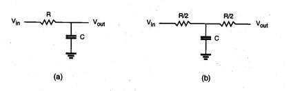
Figure 6.23. (a) Simple lumped RC model of an interconnect line, where R and C represent the total line resistance and capacitance, respectively. (b) The T-model of the same line.
