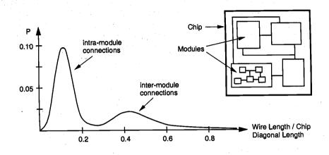
Figure 6.14. Statistical distribution of interconnection length on a typical chip.
