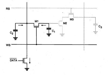
**Figure 10.42.** Both  $C_1$  and  $C_2$  are discharged via M1 and the data write transistor during the write "0" sequence.
