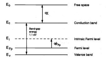
Figure 3.2. Energy band diagram of a p-type silicon substrate.
