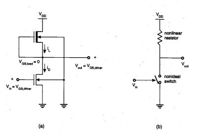
Figure 5.12. (a) Inverter circuit with depletion-type nMOS load. (b) Simplified equivalent circuit consisting of a nonlinear load resistor and a nonideal switch controlled by the input.
