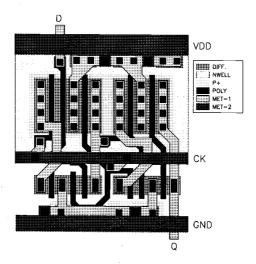
Figure 9.43. Mask layout of the TSPC-based DFF circuit.
