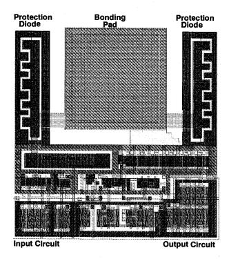
Figure 13.18. Layout of a bidirectional I/O pad circuit (courtesy of MOSIS).
