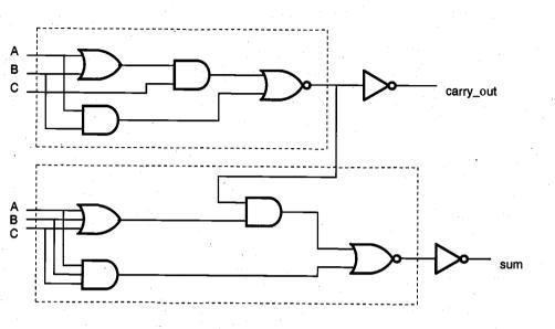
Figure 1.7. Gate-level schematic of the one-bit full-adder circuit.
