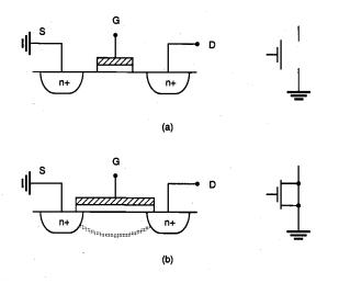
Figure 16.3. MOS transistor with (a) stuck-open (off) fault and (b) stuck-on (short) fault.
