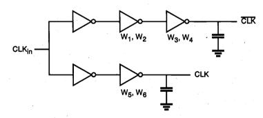
Figure 15.19. Clock distribution circuit.
