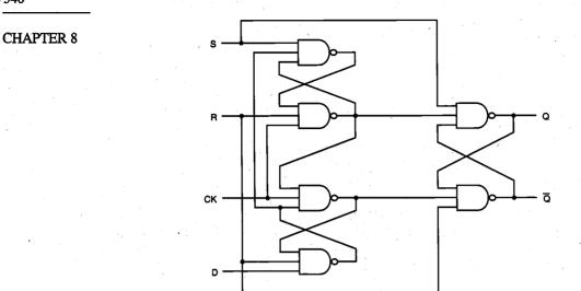
Figure 8.34. NAND3-based positive edge-triggered D flip-flop circuit.
