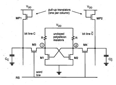
Figure 10.22. Basic structure of the resistive-load SRAM cell, shown with the column pull-up transistors.
