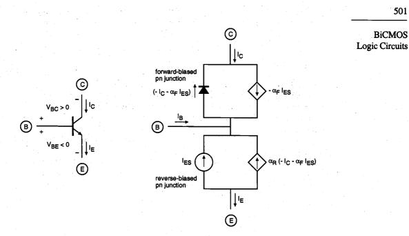
Figure 12.9. The Ebers-Moll equivalent circuit diagram of the npn BJT operating in reverse active mode.
