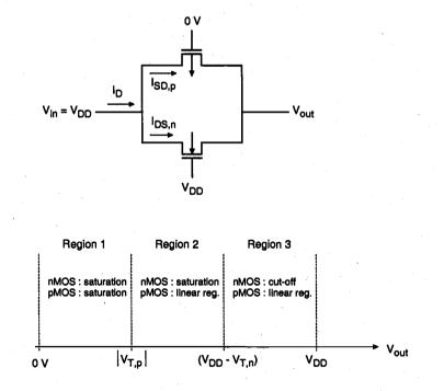
Figure 7.34. Bias conditions and operating regions of the CMOS transmission gate, shown as functions of the output voltage.
