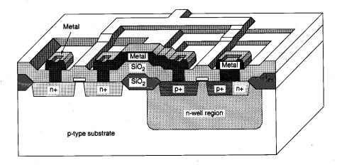
**Figure 2.10.** Metal (aluminum) is deposited over the entire chip surface using metal evaporation, and the metal lines are patterned through etching. Since the wafer surface is non-planar, the quality and the integrity of the metal lines created in this step are very critical and are ultimately essential for circuit reliability. After *Atlas of IC Technologies*, by W. Maly [1].
