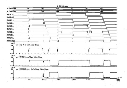
Figure 1.17. Simulated input and output waveforms of the 8-bit carry ripple adder circuit, showing a maximum signal propagation delay of about 7 ns.
