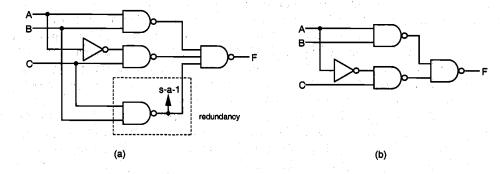
Figure 16.7. (a) A redundant logic gate example. (b) Equivalent gate with redundancy removed.
