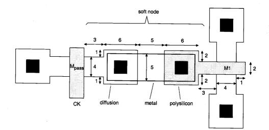
We will assume that the power supply voltage used in this circuit is  $V_{DD} = 5$  V, and that the soft node has initially been charged up to its maximum voltage,  $V_{max}$ . In order to estimate the worst-case holding time, the total soft-node capacitance must be calculated first. The simplified mask layout of the structure is shown in the following. All dimensions are given in micrometers. The critical material parameters to be used in this example are listed below.
