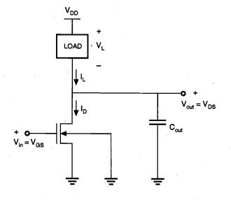
Figure 5.3. General circuit structure of an nMOS inverter.
