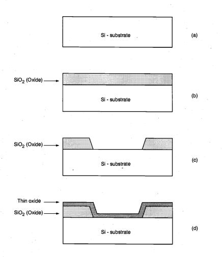
*Figure 2.4.* Process flow for the fabrication of an n-type MOSFET on p-type silicon.
