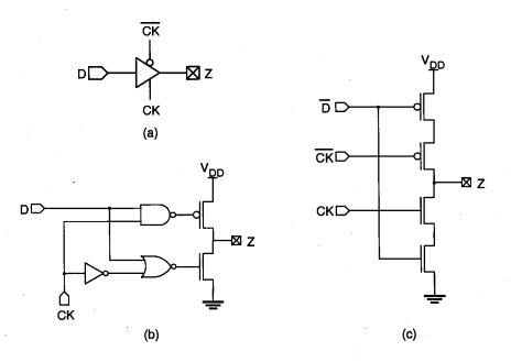
Figure 13.12. (a) Symbolic view of a tristable output circuit. (b), (c) Two different circuit implementations.
