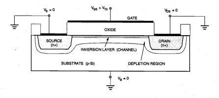
Figure 3.12. Formation of an inversion layer (channel) in an n-channel enhancement-type MOSFET.
