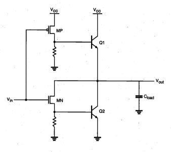
Figure 12.19. Simple BiCMOS inverter circuit with resistive base pull-down.
