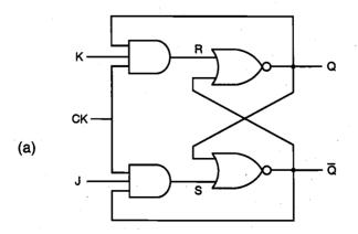
Figure 8.21. (a) Gate-level schematic of the clocked NOR-based JK latch circuit.
