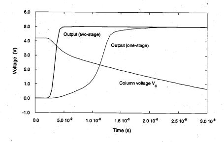
Figure 10.32. Typical dynamic response characteristics of the one-stage sense amplifier and the two-stage sense amplifier circuits.
