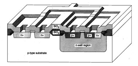
**Figure 2.9.** An insulating silicon dioxide layer is deposited over the entire wafer using CVD. Then, the contacts are defined and etched away to expose the silicon or polysilicon contact windows. These contact windows are necessary to complete the circuit interconnections using the metal layer, which is patterned in the next step. After *Atlas of IC Technologies*, by W. Maly [1].
