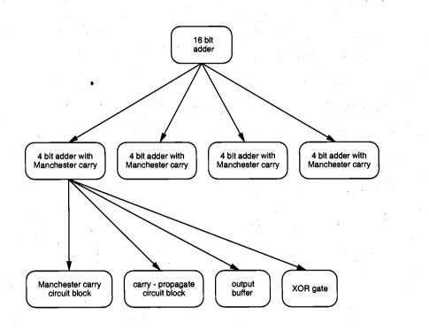
Figure 14.8. Structural hierarchy of the 16-bit adder circuit.
