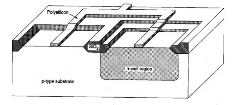
**Figure 2.7.** The polysilicon layer is deposited using chemical vapor deposition (CVD) and patterned by dry (plasma) etching. The created polysilicon lines will function as the gate electrodes of the nMOS and the pMOS transistors and their interconnects. Also, the polysilicon gates act as self-aligned masks for the source and drain implantations that follow this step. After Atlas of IC Technologies, by W. Maly [1].
