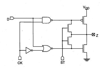
Figure 13.14. Circuit structure for reducing (di/dt) noise.
