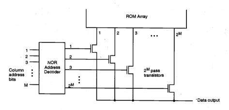
Figure 10.14. Bit-line (column) decoder arrangement using a NOR address decoder and nMOS pass transistors for every bit line.
