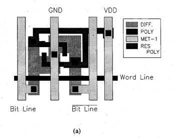
Figure 10.25. (a) Layout of the resistive-load SRAM cell.
