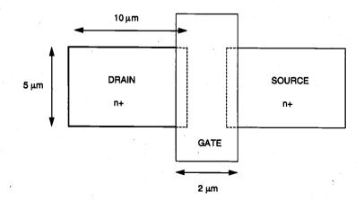
Note that both the source and the drain diffusion regions are surrounded by  $p^+$  channel-stop diffusion. The substrate is biased at 0 V. Assuming that the drain voltage is changing from 0.5 V to 5 V, find the average drain-substrate junction capacitance  $C_{dh}$ .
