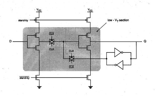
Figure 11.14. Low-power/low-voltage D-latch circuit designed with MTCMOS technique.
