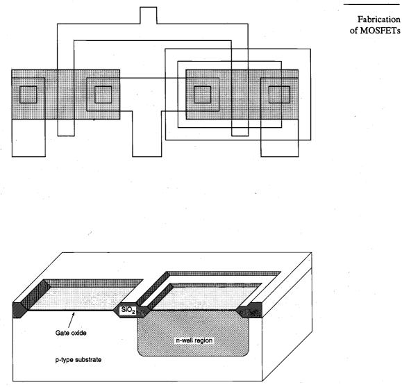
**Figure 2.6.** Following the creation of the n-well region, a thick field oxide is grown in the areas surrounding the transistor's active regions, and a thin gate oxide is grown on top of the active regions. The thickness and the quality of the gate oxide are two of the most critical fabrication parameters, since they strongly affect the operational characteristics of the MOS transistor, as well as its long-term reliability. After *Atlas of IC Technologies*, by W. Maly [1].
