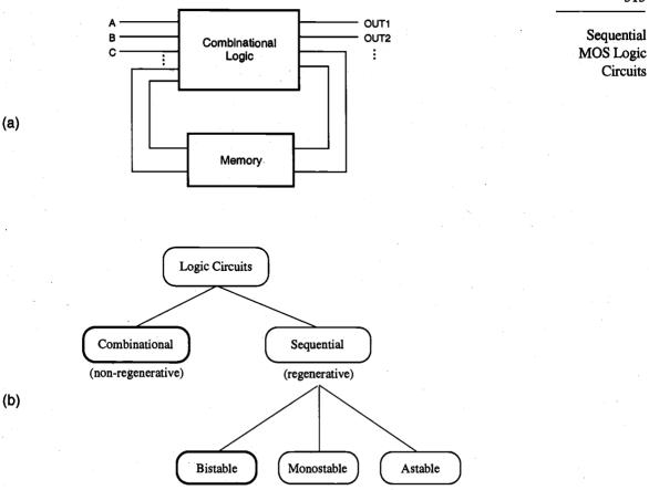
Figure 8.1. (a) Sequential circuit consisting of a combinational logic block and a memory block in the feedback loop. (b) Classification of logic circuits based on their temporal behavior.
