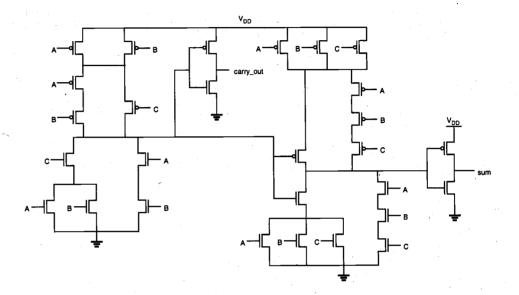
Figure 1.8. Transistor-level schematic of the one-bit full-adder circuit.
