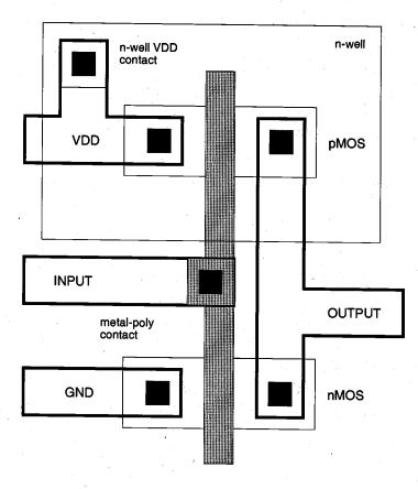
Figure 2.16. Complete mask layout of the CMOS inverter.
