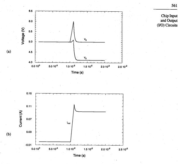
Figure 13.31. Simulated (a) voltage and (b) current waveforms of the CMOS inverter circuit during latch-up triggered through the output node.
