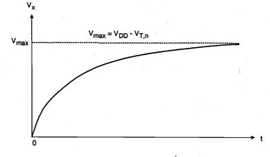
Figure 9.3. Variation of  $V_r$  as a function of time during logic "1" transfer.
