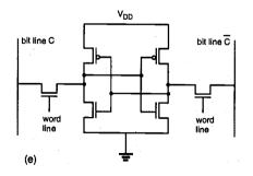
*Figure 10.21.* Various configurations of the static RAM cell. (a) Symbolic representation of the two-inverter latch circuit with access switches. (b) Generic circuit topology of the MOS static RAM cell. (c) Resistive-load SRAM cell. (d) Depletion-load nMOS SRAM cell. (e) Full CMOS SRAM cell.
