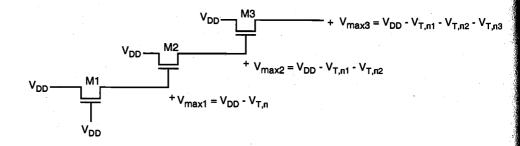
*Figure 9.5.* Node voltages during the logic "1" transfer, when each pass transistor is driving another pass transistor.
