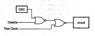
Figure 16.6. Avoid synchronization problems via disabling of the oscillator.
