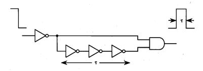
Figure 16.8. A pulse-generation circuit using a delay chain of three inverters.
