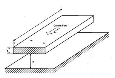
Figure 6.16. Interconnect segment running parallel to the surface, which is used for parasitic resistance and capacitance estimations.
