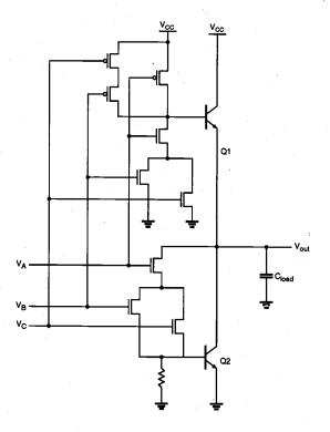
Figure 12.32. Circuit diagram of a BiCMOS complex logic gate.
