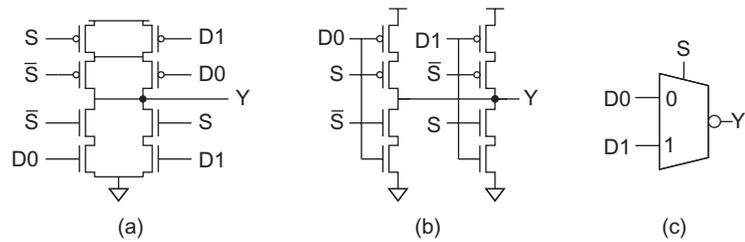
FIGURE 1.29 Inverting multiplexer
