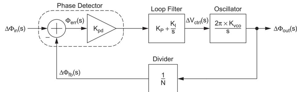
FIGURE 13.34 Linear system model of a PLL
