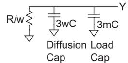
FIGURE 4.13 Equivalent circuit for wider inverter
