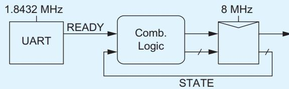
**FIGURE 10.53** Unsynchronized input
