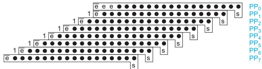
**FIGURE 11.83** Radix-4 Booth-encoded partial products for signed multiplication
