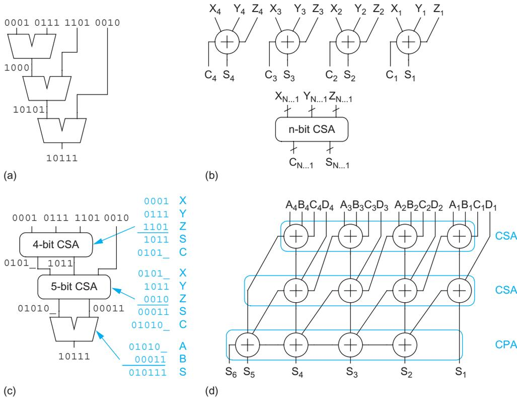
FIGURE 11.42 Multiple-input adders
