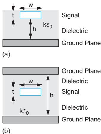
**FIGURE 13.56** Transmission lines
