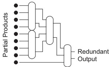
**FIGURE 11.86** Dot diagram for [4:2] tree multiplier
