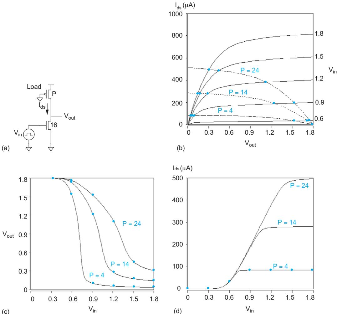
**FIG 9.13** Pseudo-nMOS inverter and DC transfer characteristics
