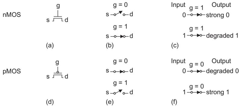
FIGURE 1.20 Pass transistor strong and degraded outputs
