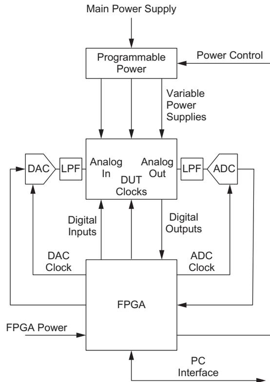
FIGURE 15.23 FPGA-assisted testing
