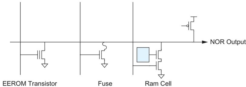
**FIGURE 14.14** PLA NOR structure (one plane shown)
