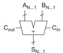
FIGURE 11.9 Carry-propagate adder
