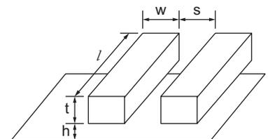
FIGURE 6.1 Interconnect geometry
