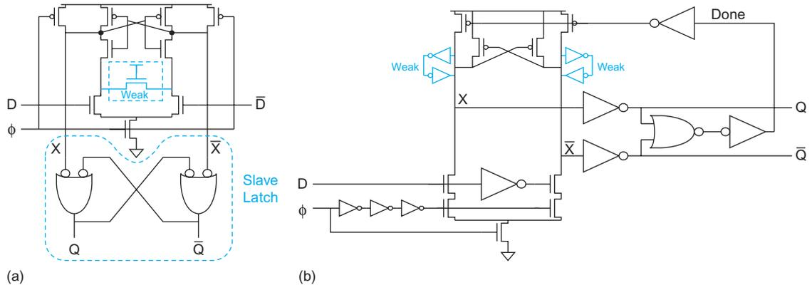
FIGURE 10.29 Differential flip-flops
