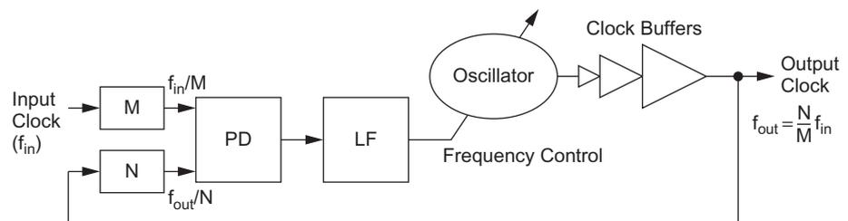
**FIGURE 13.23** Frequency multiplication using a PLL
