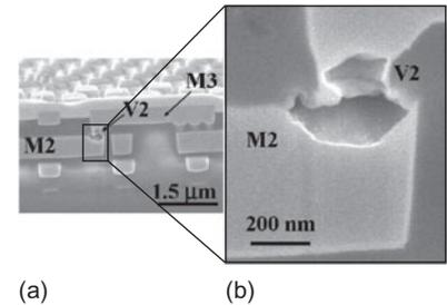
FIGURE 7.8 Electromigration failure of M2-M3 via (© IEEE 2006.)
