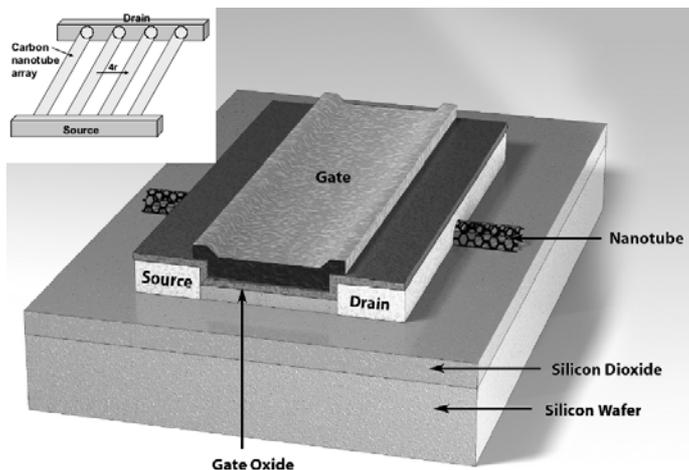
**FIGURE 3.35** Carbon nanotube transistor (© IEEE 2003.)
