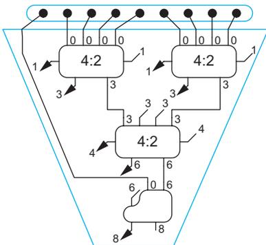
FIGURE 11.93 Vertical compressor slice using [4:2] compressors
