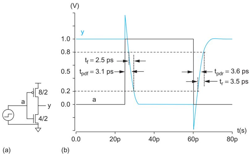
FIGURE 8.7 Unloaded inverter
