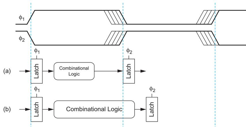
FIGURE 10.34 Latch placement and time borrowing
