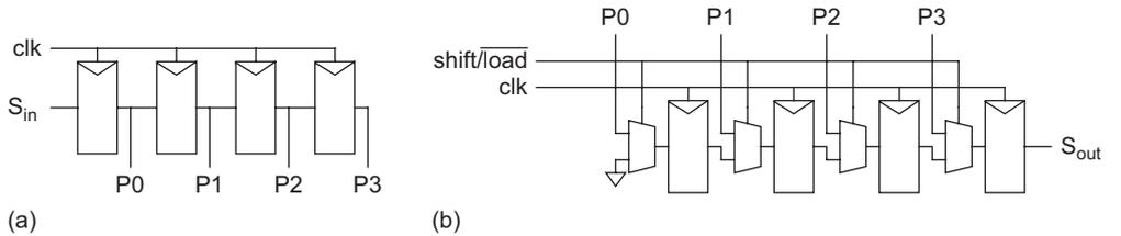
FIGURE 12.65 Serial/parallel memories
