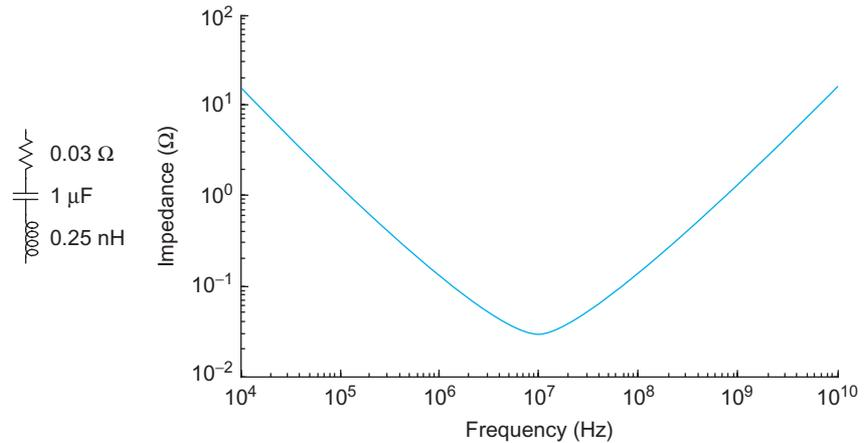
**FIGURE 13.11** Impedance of bypass capacitor
