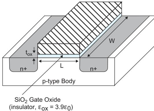
FIGURE 2.6 Transistor dimensions
