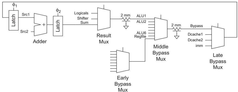
FIGURE 10.14 ALU self-bypass path with two-phase latches
