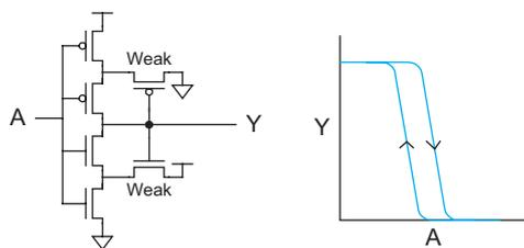
**FIGURE 13.46** Schmitt trigger
