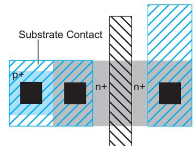
**FIGURE 3.16** Substrate contact
