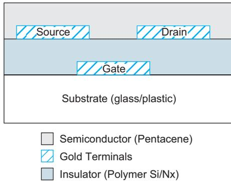
FIGURE 3.20 Plastic transistors
