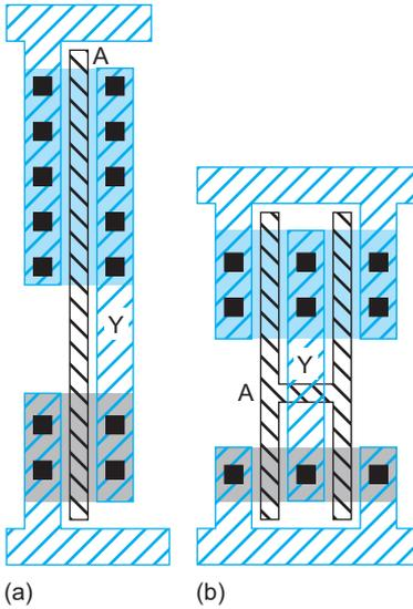
**FIGURE 4.18** Layout styles: (a) conventional, (b) folded
