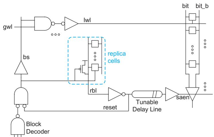
FIGURE 12.30 Replica delay for sense amplifier enable
