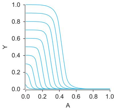
**FIGURE 9.66** Inverter DC transfer characteristics at low voltage
