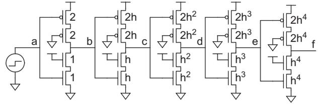
FIGURE 8.27 Circuit for extracting effective series resistance
