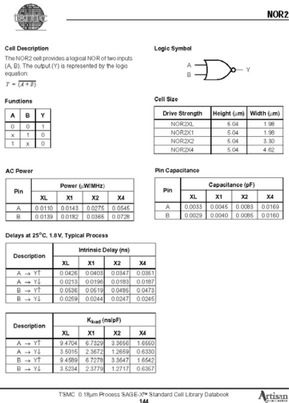
**FIGURE 4.41** 2-input NOR datasheet (Courtesy of Artisan Components.)
