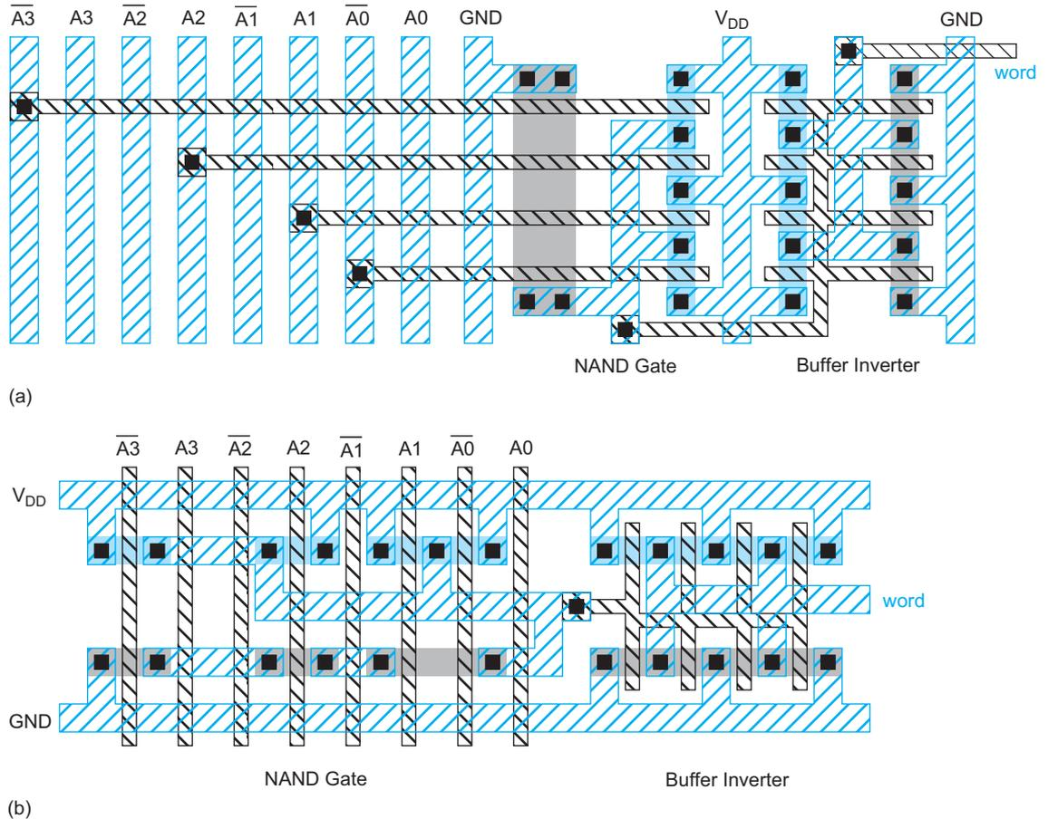
FIGURE 12.22 Stick diagrams of two decoder layouts
