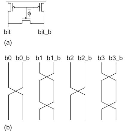
FIGURE 12.29 Bitline noise reduction through equalizers and twisting
