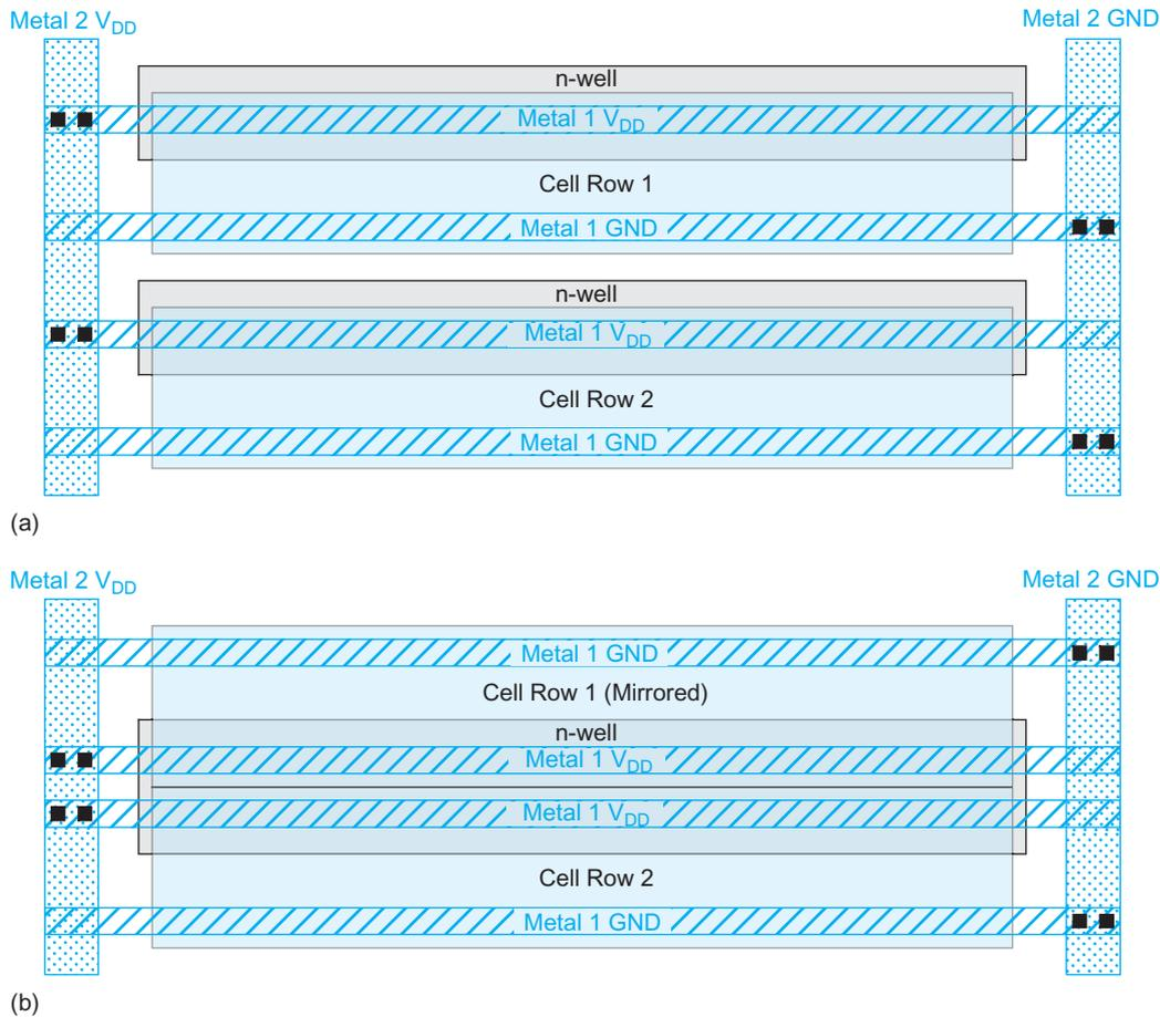
**FIGURE 13.7** Power distribution for standard cell layout
