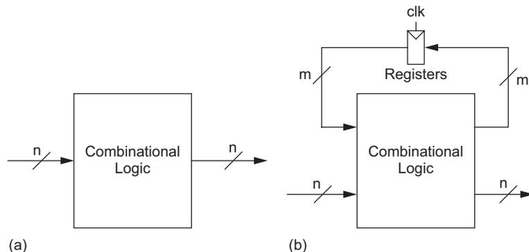
**FIGURE 15.6** The combinational explosion in test vectors
