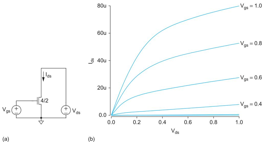
**FIGURE 8.5** MOS I-V characteristics. Current in units of microamps (u).
