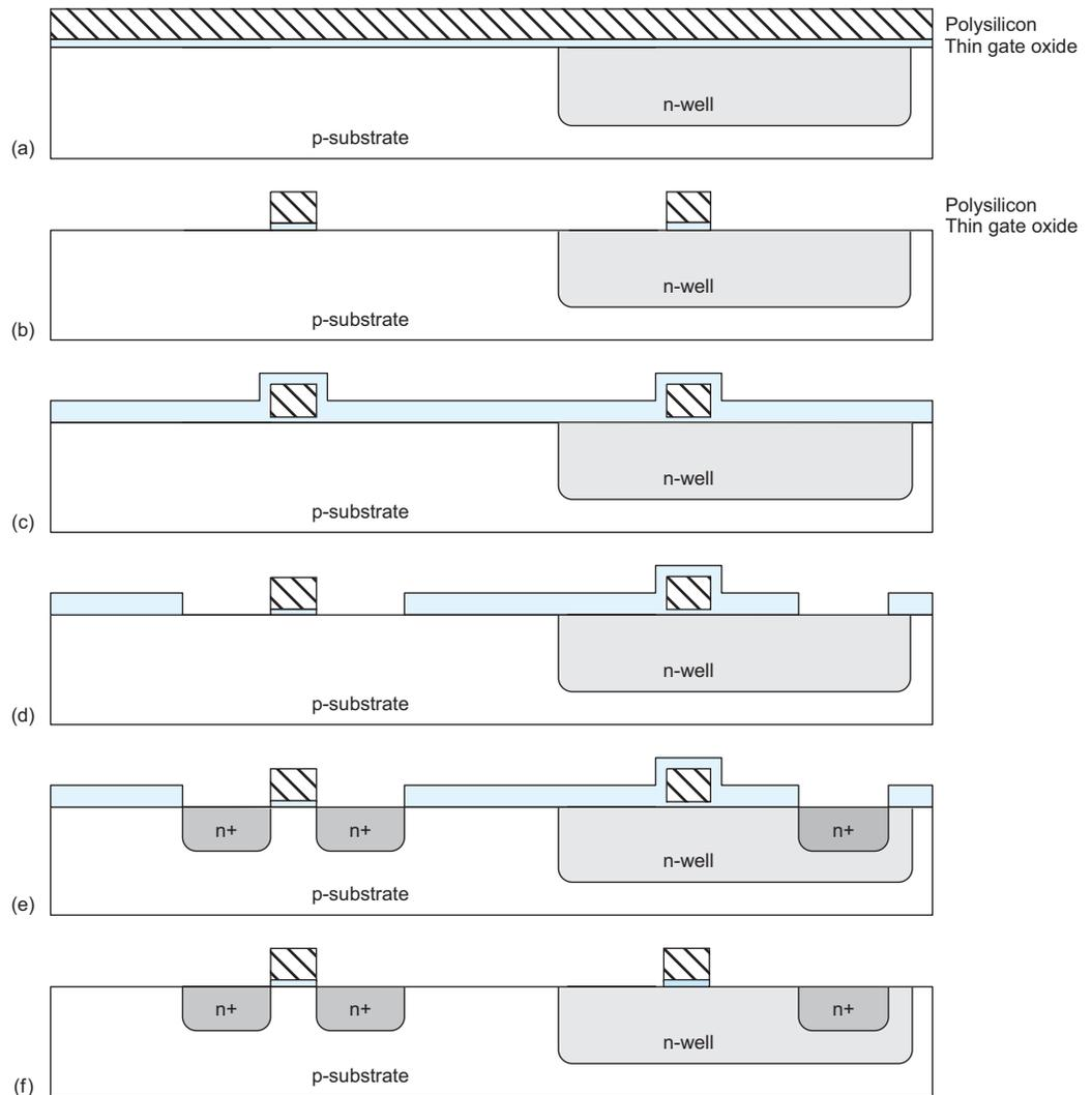
**FIGURE 1.37** Cross-sections while manufacturing polysilicon and n-diffusion
