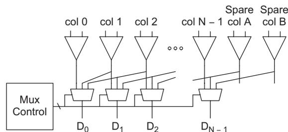
**FIGURE 12.81** Column redundancy
