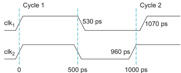
FIGURE 13.19 Skewed clock waveforms
