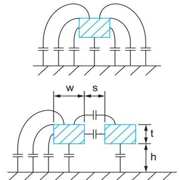
FIGURE 6.9 Effect of fringing fields on capacitance
