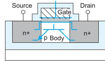
FIGURE 9.64 Parasitic bipolar transistor in PD SOI
