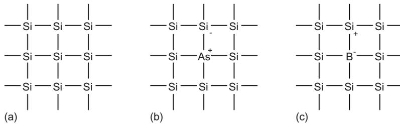
FIGURE 1.7 Silicon lattice and dopant atoms
