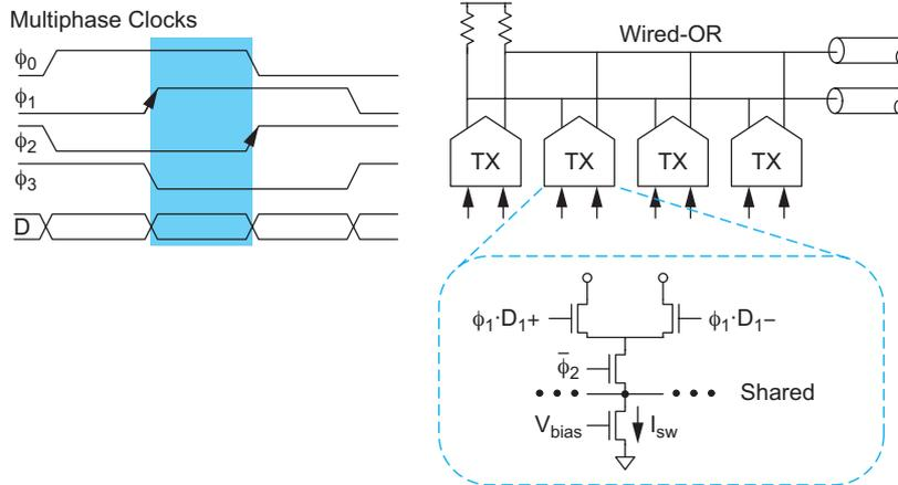
FIGURE 13.67 Time-interleaved transmitter
