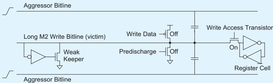
FIGURE 15.25 Register file write circuitry
