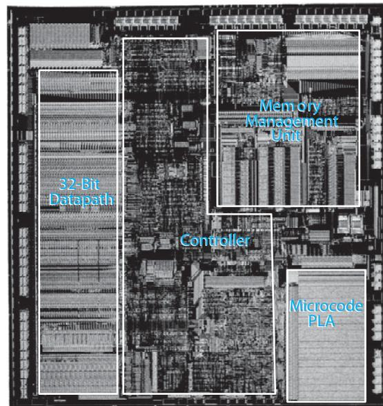
**FIGURE 7.32** Intel386 microprocessor (Courtesy of Intel Corporation.)
