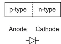
FIGURE 1.8 *p*-*n* junction diode structure and symbol
