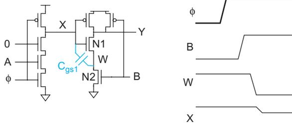
FIGURE 9.59 Back-gate coupling
