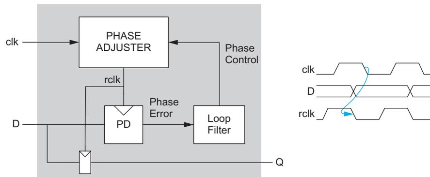
FIGURE 13.74 Phase calibration loop for mesochronous timing recovery
