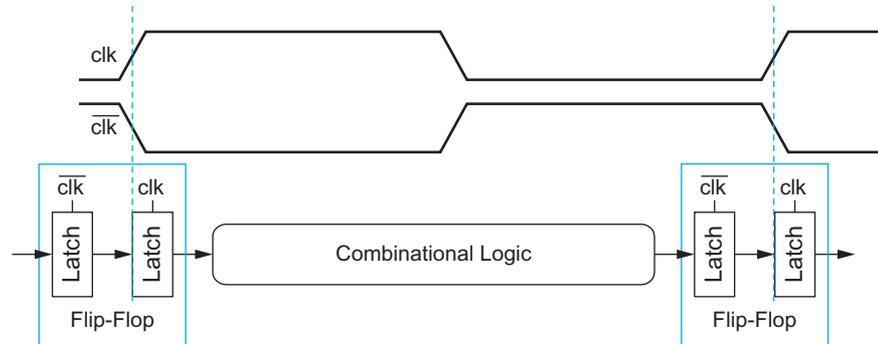
FIGURE 10.3 Flip-flop viewed as back-to-back latch pair
