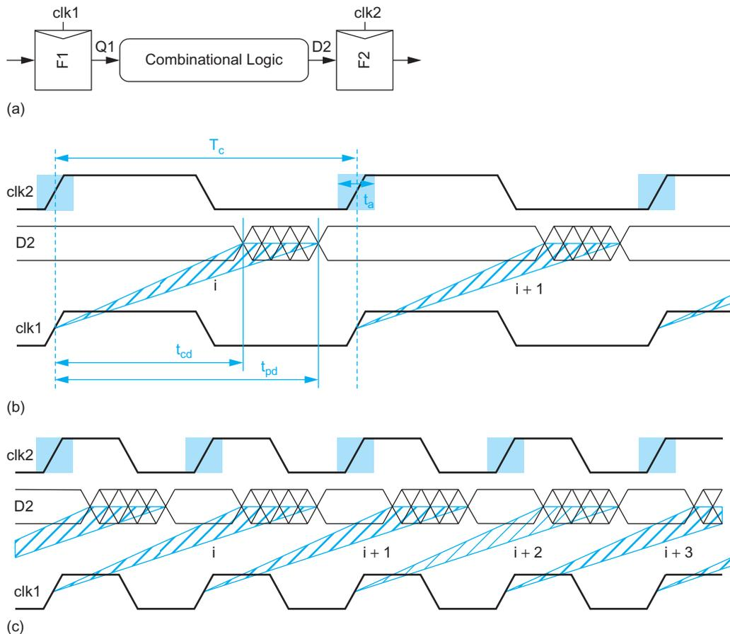
FIGURE 10.52 Wave pipelining
