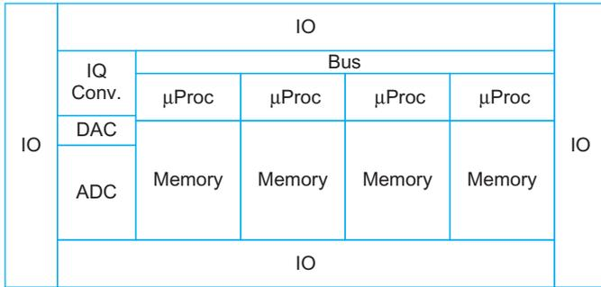
FIGURE 14.12 A possible floorplan for software radio
