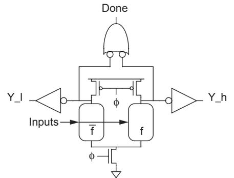
**FIGURE 9.31** Dual-rail domino gate with completion detection
