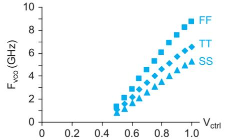
FIGURE 13.36 VCO voltage-to-frequency characteristics over different process conditions
