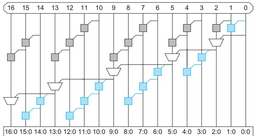
**FIGURE 11.19** Variable group size carry-skip adder PG network
