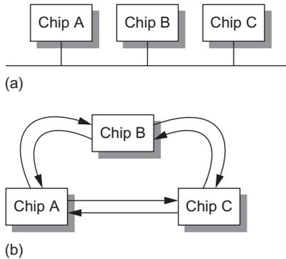
**FIGURE 13.58** (a) multidrop bus vs. (b) point-to-point links
