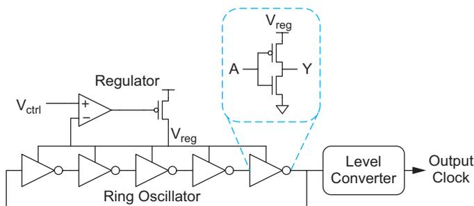
**FIGURE 13.35** Voltage-controlled oscillator
