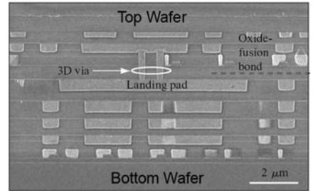
**FIGURE 3.32** Scanning electron micrograph of 3-dimensional integration of two wafers (Reprinted from [Koester08]. Courtesy of International Business Machines Corporation. Unauthorized use not permitted.)
