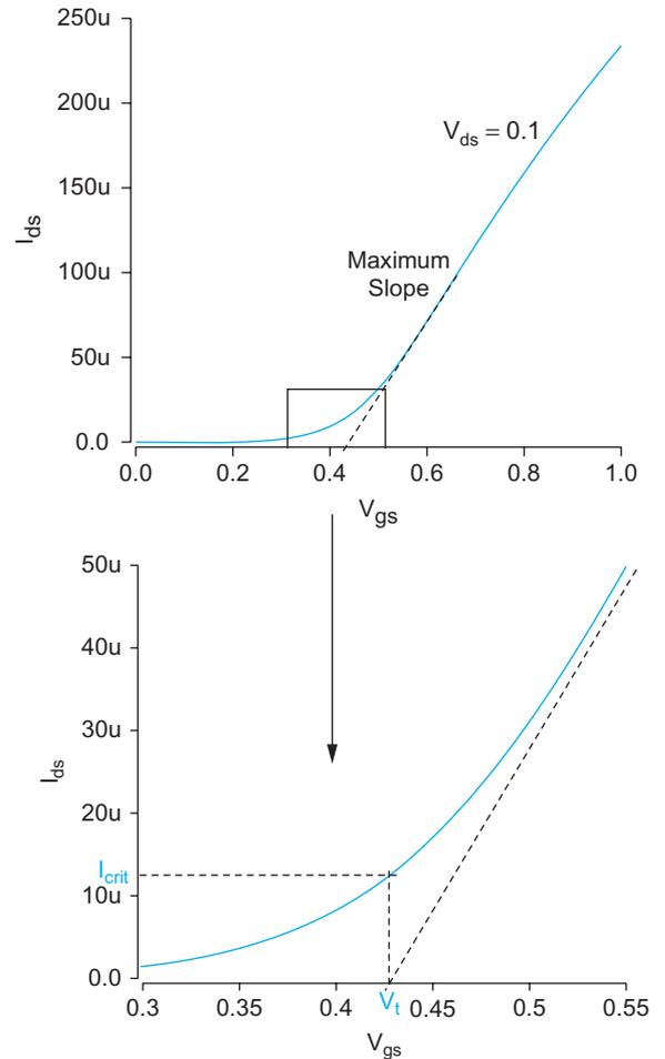
**FIGURE 8.20** Linear extrapolation threshold voltage extraction method
