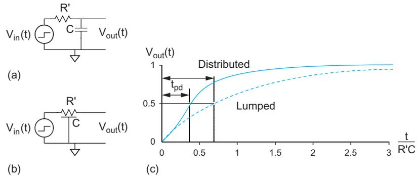
**FIGURE 6.24** Lumped and distributed RC circuit response
