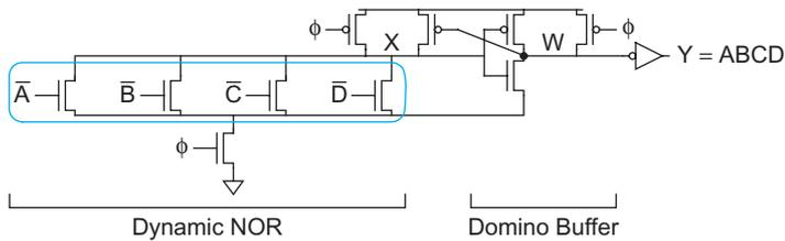
FIGURE 12.25 4-input AND using race-based NOR
