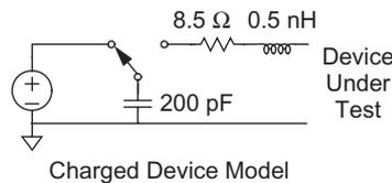
capacitor to the pin through a resistor and/or inductor. The *human body model* (HBM) represents the discharge that takes place when an ungrounded person touches a pin of the chip. The *charged device model* (CDM) represents the pin *triboelectrically* charging during manufacturing (i.e., charging through contact with a different material) and then rapidly discharging when it comes in contact with a grounded conductor. The CDM zap is more difficult to protect against, but is also
