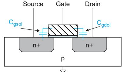
**FIGURE 2.10** Overlap capacitance
