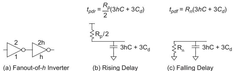
**FIGURE 8.26** RC delay model for fanout-of- $h$  inverter
