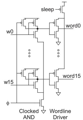
**FIGURE 12.21** Shared clock and transistors in wordline driver
