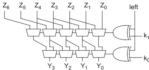
**FIGURE 11.64** 4-bit logarithmic funnel shifter
