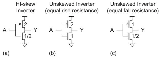
FIGURE 9.9 Logical effort calculation for HI-skew inverter
