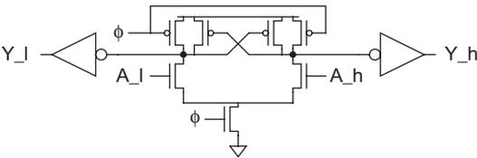
FIGURE 9.35 Differential keeper
