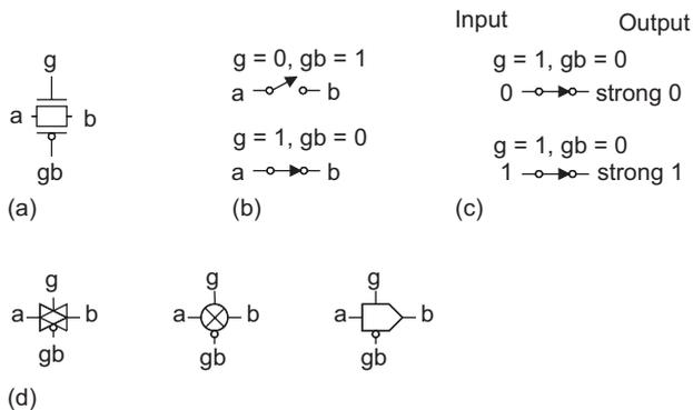
FIGURE 1.21 Transmission gate
