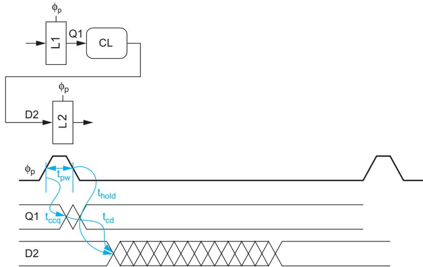
FIGURE 10.11 Pulsed latch min-delay constraint
