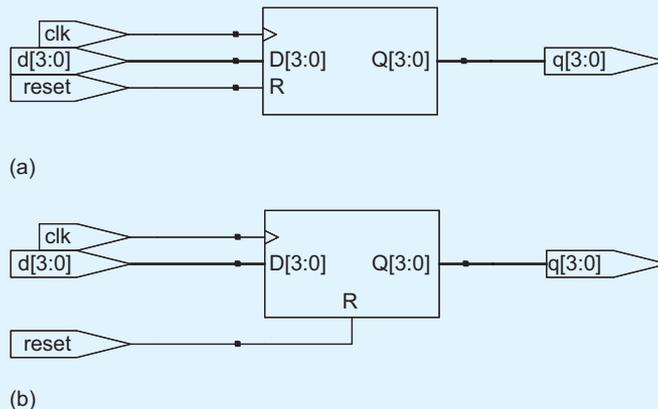
**FIGURE A.18** flop\_r (a) synchronous reset, (b) asynchronous reset
