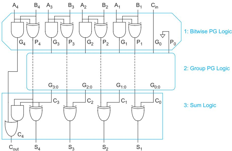
FIGURE 11.12 Addition with generate and propagate logic
