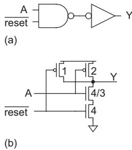
**FIGURE 9.7** Resettable buffer optimized for data input
