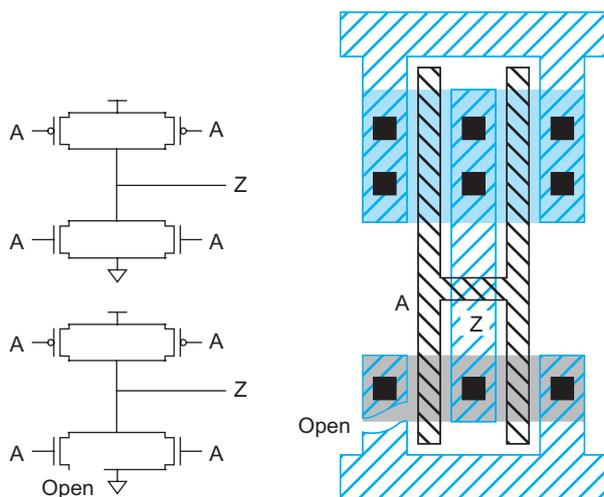
FIGURE 15.15 An example of a delay fault
