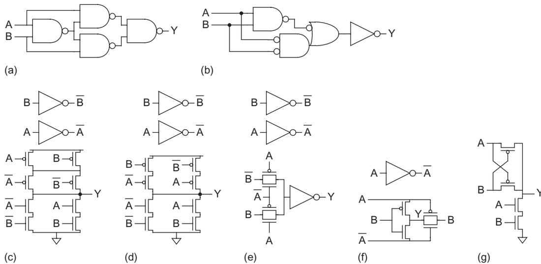
FIGURE 11.59 Static 2-input XOR designs
