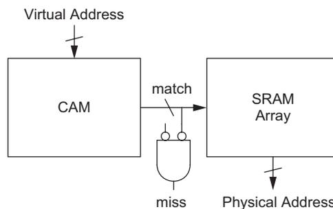
FIGURE 12.68 Translation Lookaside Buffer (TLB) using CAM
