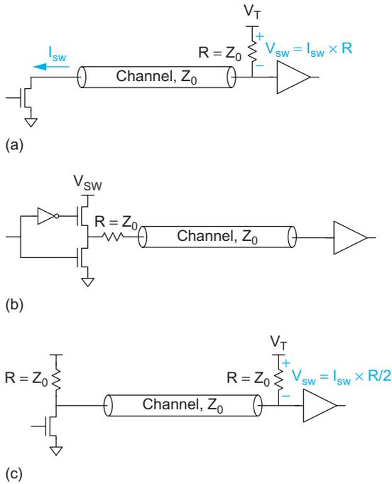
**FIGURE 13.61** Transmission line drivers (a) current-mode driver (parallel termination at the receiving end), (b) voltage-mode driver (series termination at the transmitting end), (c) double-terminated driver (distinction between voltage and current is irrelevant)
