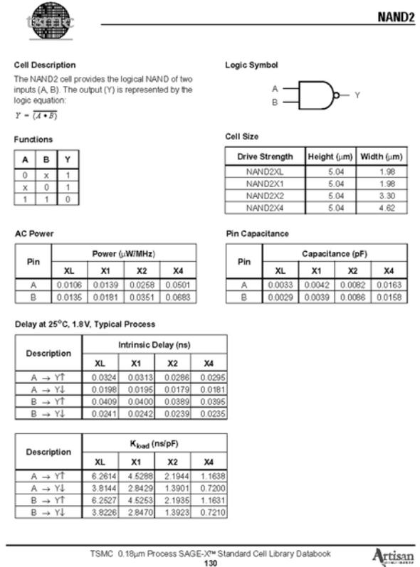
Figure 4.25 Artisan Components cell library datasheets. Reprinted with permission.
