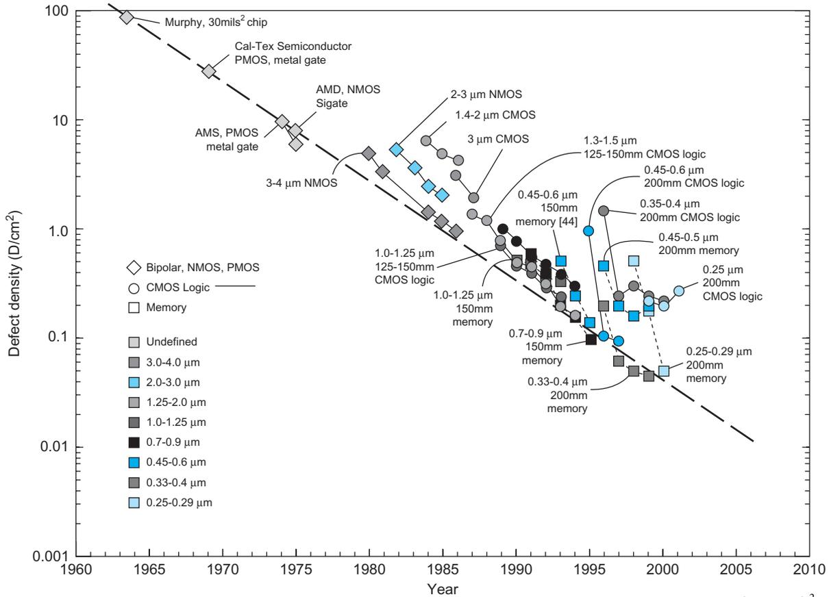
**FIGURE 14.27** Defect density trends. Note that this data uses the Murphy Model rather than the Poisson Model:  $Y = \left( \frac{1 - e^{-AD}}{AD} \right)^2$ . The Murphy Model predicts better yield at high defect density. (© 2002 IC Knowledge LLC, www.icknowledge.com reprinted with permission.)
