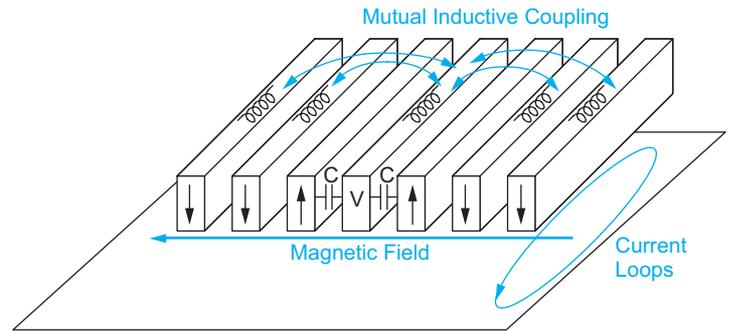
FIGURE 6.23 Inductive and capacitive crosstalk in a bus
