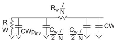
FIGURE 6.27 Equivalent circuit for segment of repeated wire
