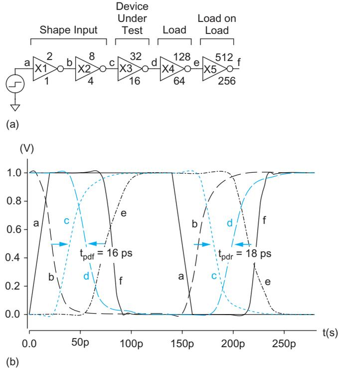
FIGURE 8.9 Fanout-of-4 inverters
