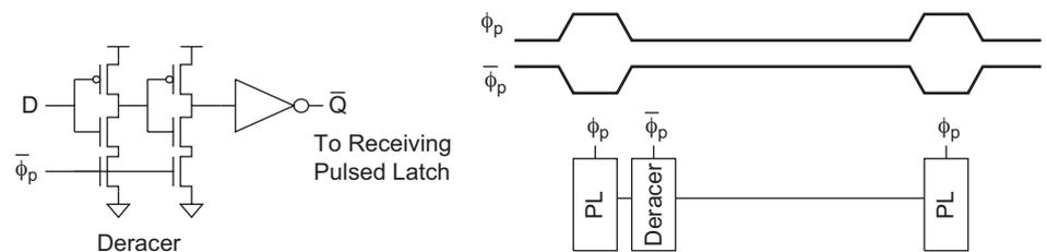
FIGURE 10.33 Clocked deracer
