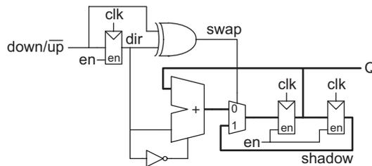
FIGURE 11.52 Fast binary up/down counter (most significant segment)
