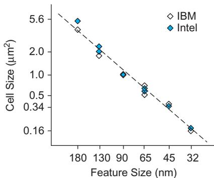
FIGURE 12.17 SRAM cell size vs. feature size
