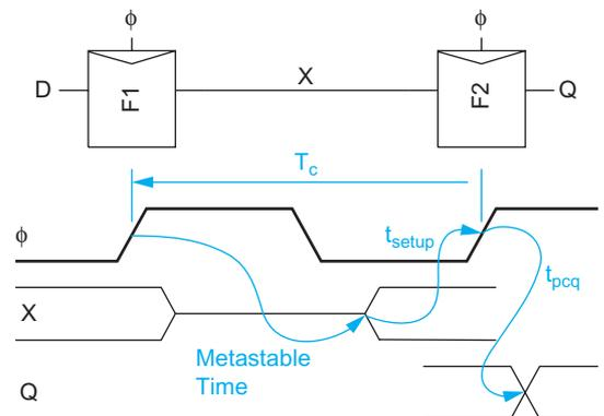
FIGURE 10.46 Simple synchronizer
