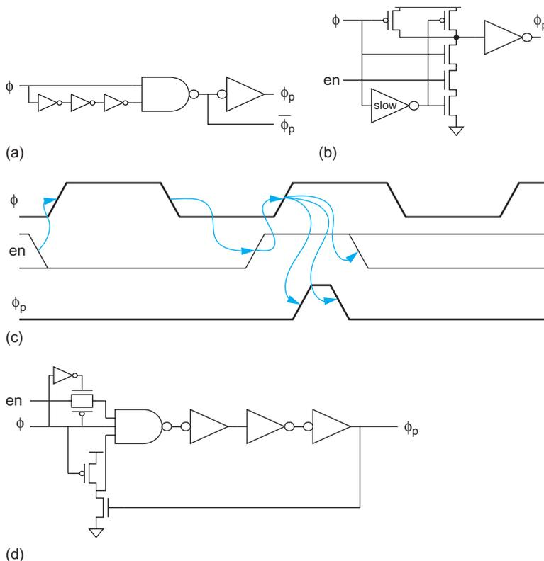
**FIGURE 10.22** Pulse generators
