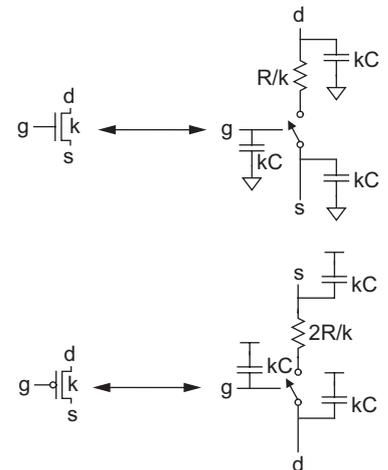
FIGURE 4.5 Equivalent circuits for transistors
