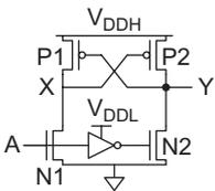
**FIGURE 5.15** Level converter
