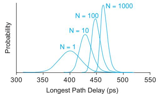
**FIGURE 7.19** Delay distributions of typical and longest paths**TABLE 7.9** Behavior of maximum of normal variables
