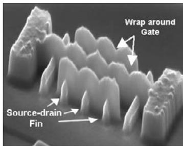
**FIGURE 3.34** Trigate transistor
