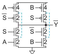
FIGURE 9.52 Logical effort of transmission gate circuit
