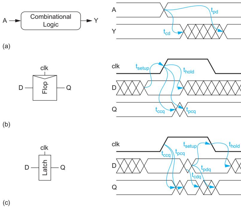
FIGURE 10.4 Timing diagrams
