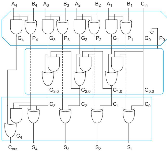
FIGURE 11.14 4-bit carry-ripple adder using PG logic
