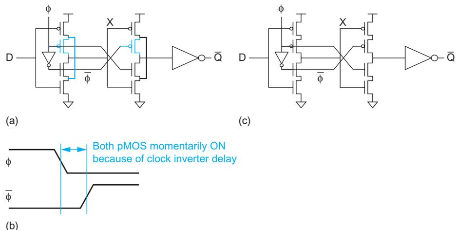
**FIGURE 10.20** Transmission gate and NORA dynamic flip-flops
