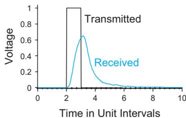
**FIGURE 13.59** Pulse dispersion due to frequency-dependent attenuation
