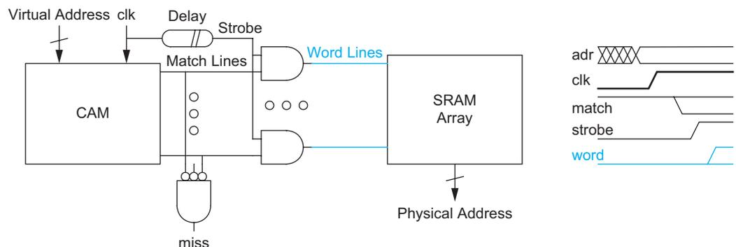
FIGURE 12.71 Refined TLB path with monotonic wordlines
