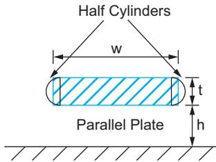
**FIGURE 6.10** Yuan & Trick capacitance model including fringing fields
