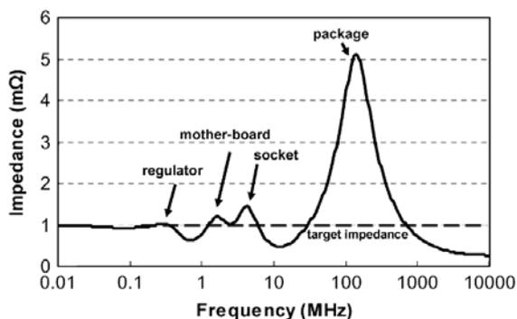
**FIGURE 13.12** Pentium 4 simulated power supply impedance (© 2008 IEEE.)
