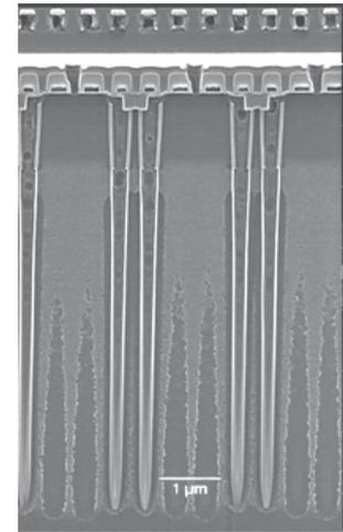
FIGURE 12.42 Trench capacitor
