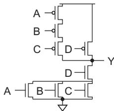
**FIGURE 1.19** CMOS compound gate for function  $Y = \overline{(A + B + C) \cdot D}$
