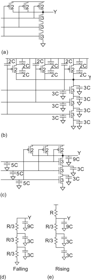
FIGURE 4.7 Equivalent circuits for a 3-input NAND gate
