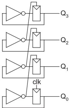
FIGURE 11.48 Asynchronous ripple-carry counter
