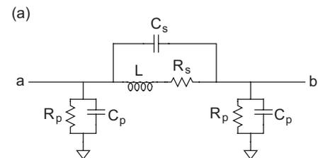
FIGURE 3.25 Typical spiral inductor and equivalent circuit [Rotella02]
