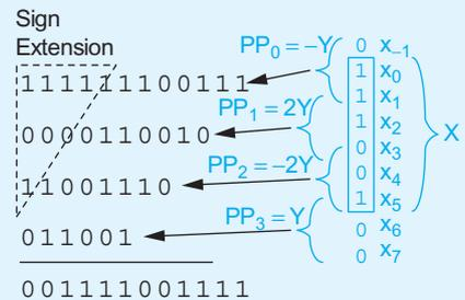
FIGURE 11.79 Booth-encoded example
