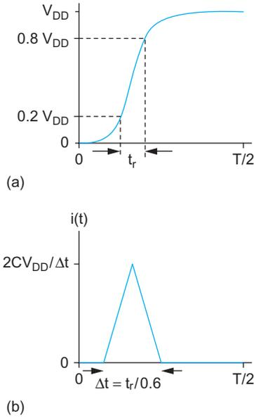
**FIGURE 7.9** Switching waveforms for RMS current estimation
