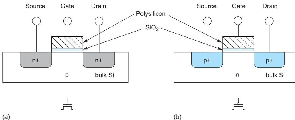
FIGURE 1.9 *nMOS* transistor (a) and *pMOS* transistor (b)
