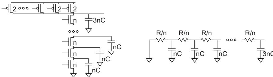
**FIGURE 4.23**  $n$ -input NAND gate parasitic delay
