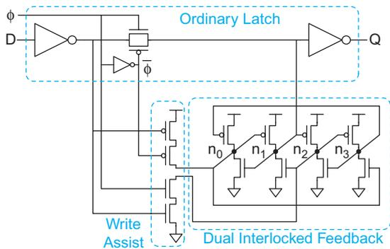
FIGURE 10.32 Radiation-hardened latch
