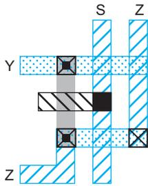
**FIGURE 11.63** Array funnel shifter cell stick diagram
