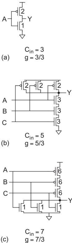
**FIGURE 4.22** Logic gates sized for unit resistance
