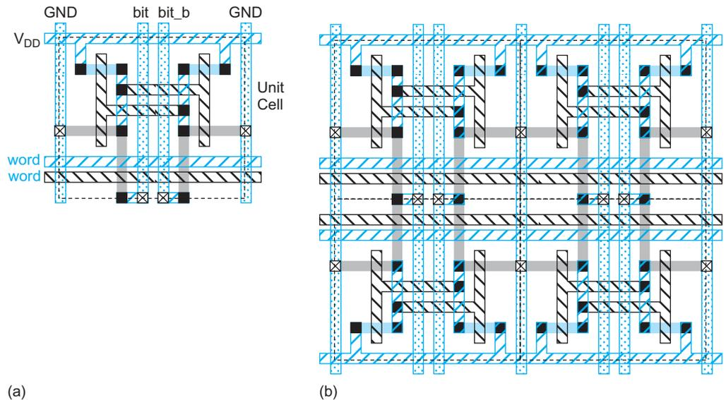
FIGURE 12.13 Stick diagram of 6T SRAM cell
