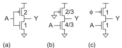
FIGURE 9.21 Comparison of (a) static CMOS, (b) pseudo-nMOS, and (c) dynamic inverters
