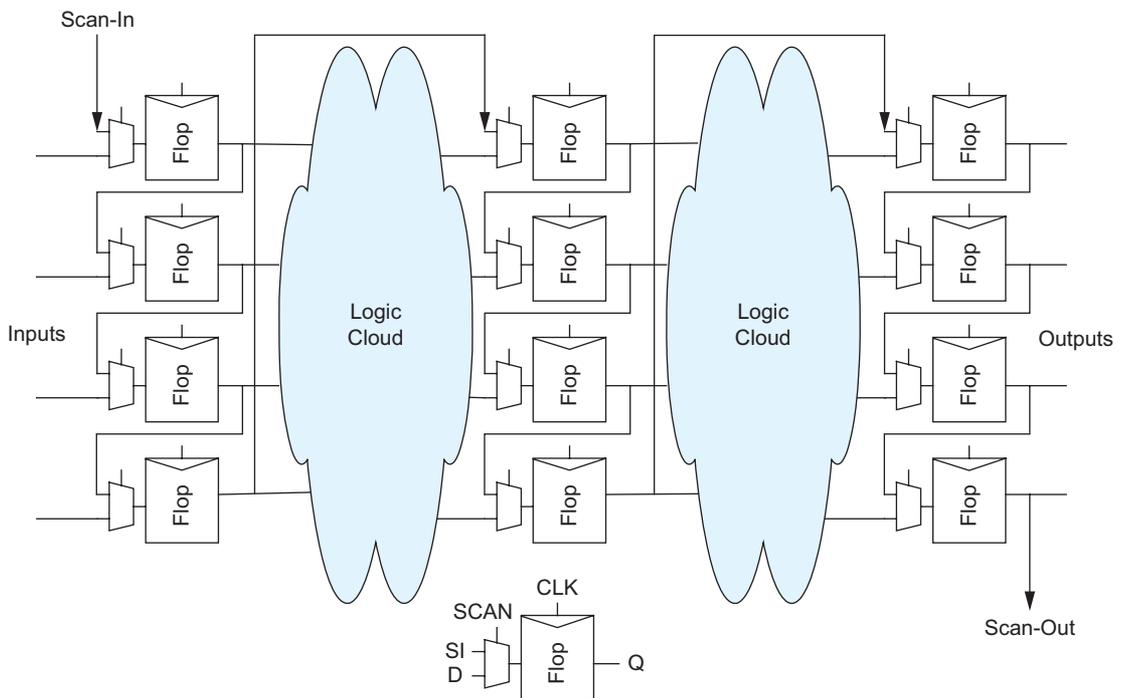
FIGURE 15.16 Scan-based testing
