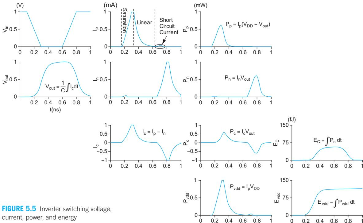
FIGURE 5.5 Inverter switching voltage, current, power, and energy
