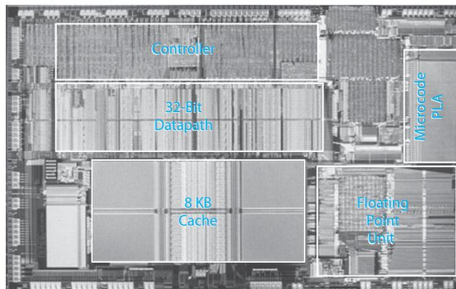
**FIGURE 7.33** Intel486 microprocessor (Courtesy of Intel Corporation.)
