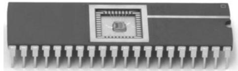
**FIGURE 1.73** Chip in a 40-pin dual-inline package
