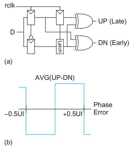
FIGURE 13.76 (a) Alexander detector, (b) transfer curves
