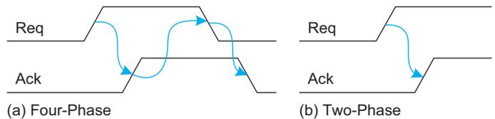
FIGURE 10.48 Four-phase and two-phase handshake protocols
