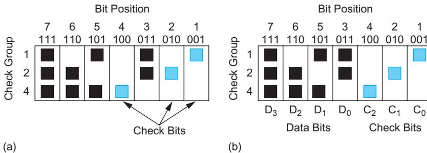
FIGURE 11.58 Parity-check matrix
