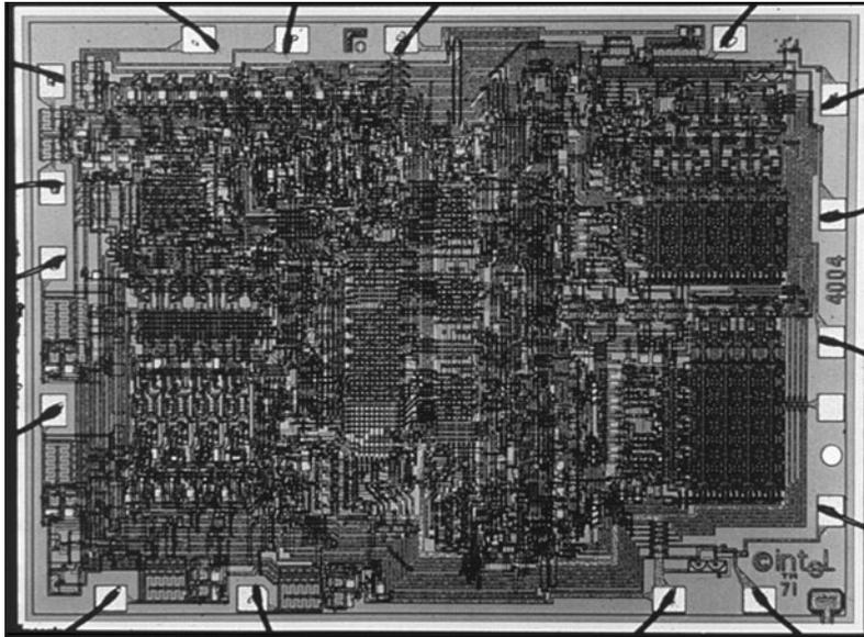
**FIGURE 7.30** 4004 microprocessor (Courtesy of Intel Corporation.)
