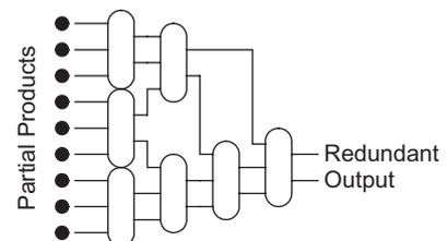
**FIGURE 11.85** Dot diagram for Wallace tree multiplier
