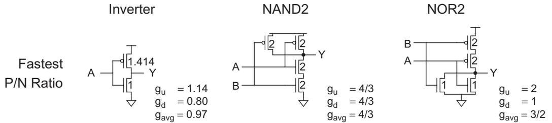
FIGURE 9.11 Gates with  $P/N$  ratios giving least delay
