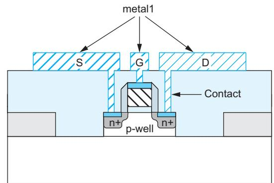
FIGURE 3.11 Aluminum metallization
