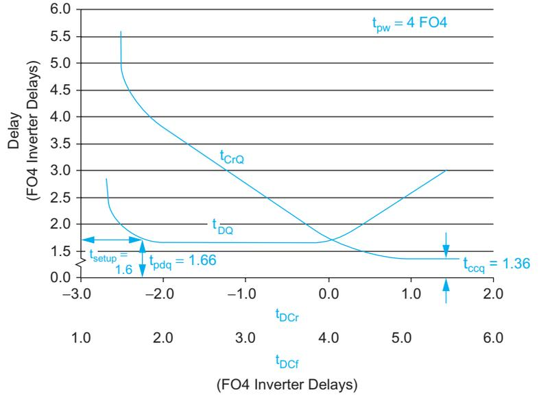
FIGURE 10.37 Latch delay vs. data arrival time
