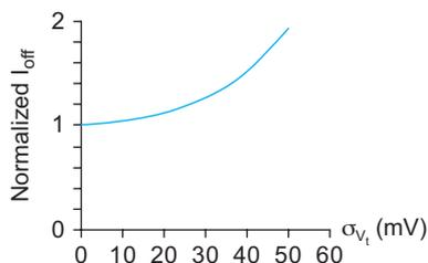
**FIGURE 7.26** Impact of random threshold voltage on average leakage
