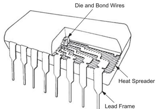
**FIGURE 13.2** Cutaway view of dual-in-line package (© IEEE 1985.)
