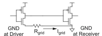
FIGURE 9.57 Power supply IR drops
