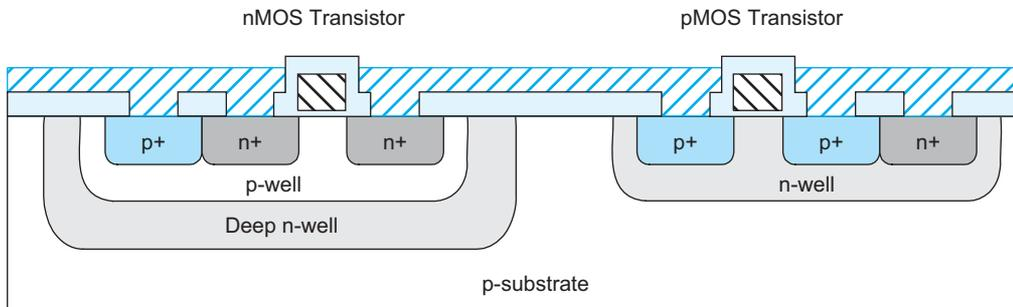
**FIGURE 3.5** Well structure in triple-well process
