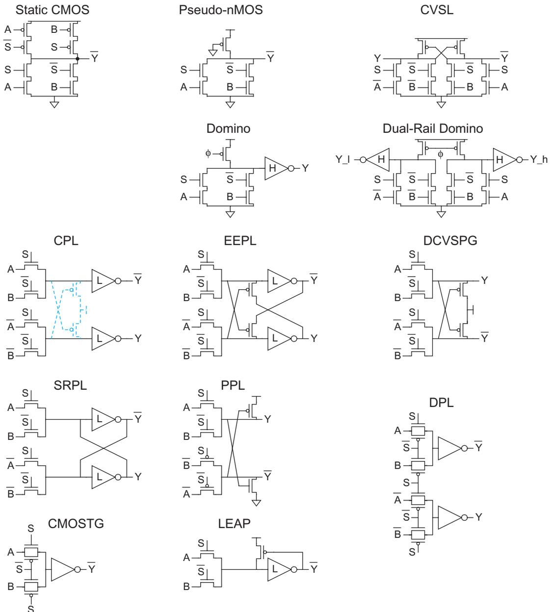
FIGURE 9.47 Comparison of circuit families for 2-input multiplexers
