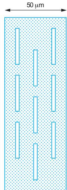
**FIGURE 3.37** Slots in wide metal power bus
