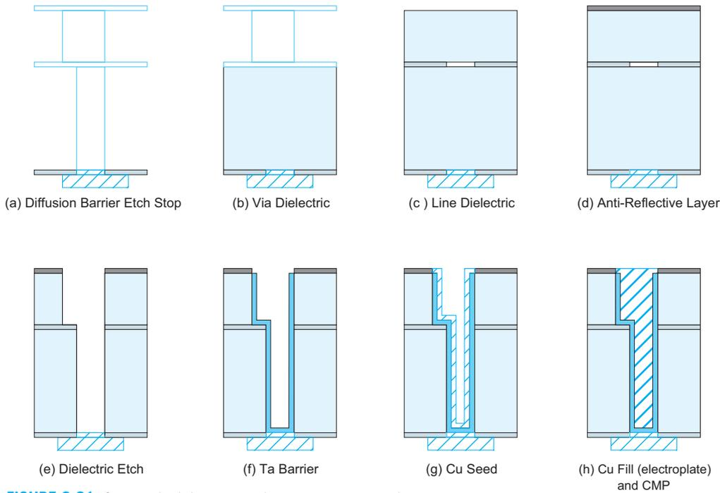
**FIGURE 3.21** Copper dual damascene interconnect processing steps
