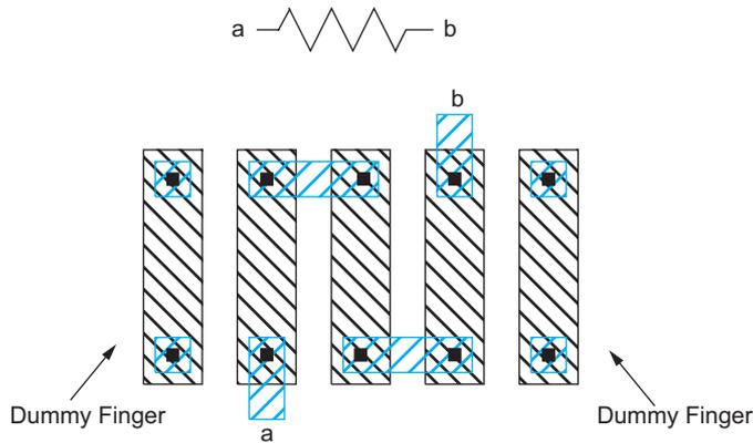
FIGURE 3.24 Resistor layout
