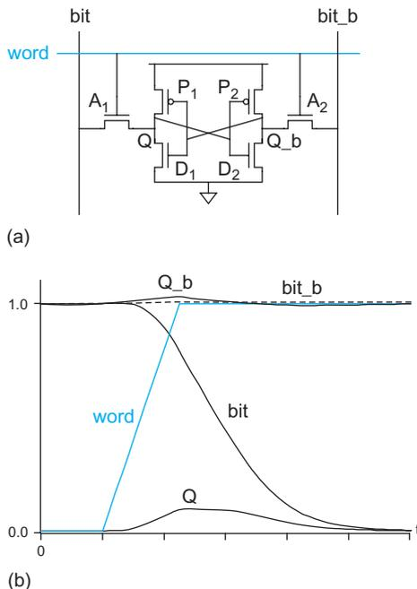
FIGURE 12.4 Read operation for 6T SRAM cell
