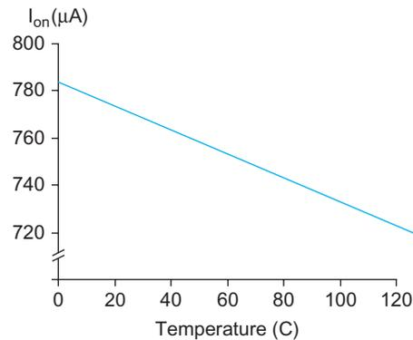
**FIGURE 2.24**  $I_{\text{dsat}}$  vs. temperature
