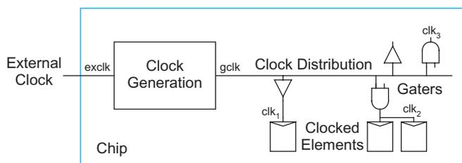
FIGURE 13.21 Clock subsystem
