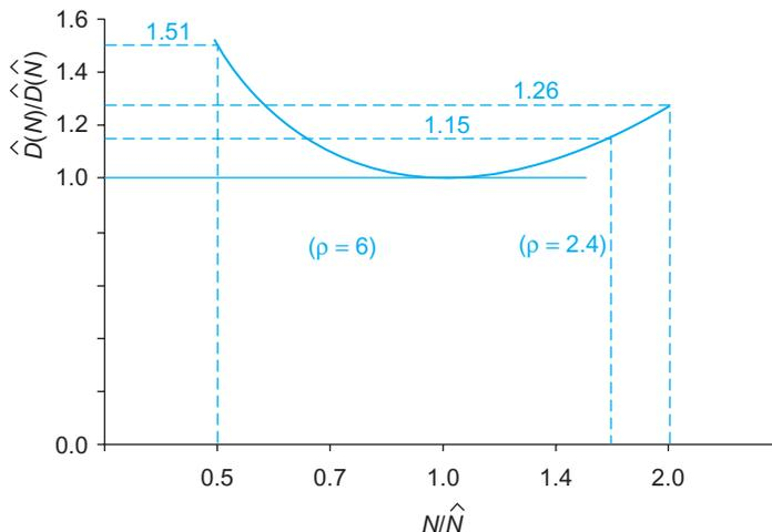
FIGURE 4.35 Sensitivity of delay to number of stages
