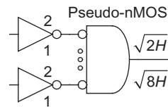
FIGURE 9.16  $k$ -input AND marked with transistor widths
