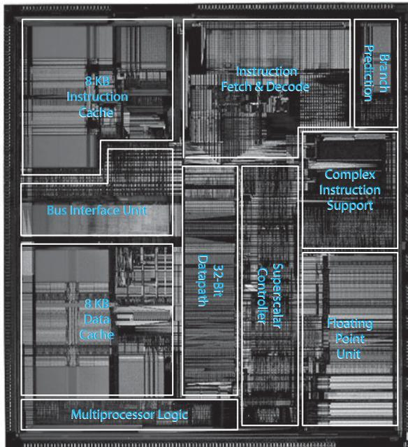
**FIGURE 7.34** Pentium microprocessor (Courtesy of Intel Corporation.)
