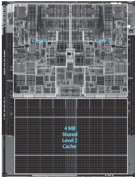
FIGURE 7.37 Core 2 Duo (Courtesy of Intel Corporation.)
