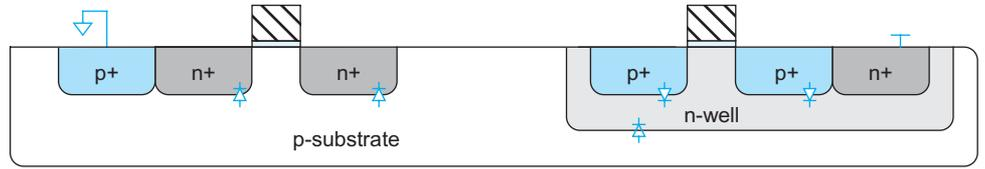
**FIGURE 2.22** Substrate to diffusion diodes in CMOS circuits
