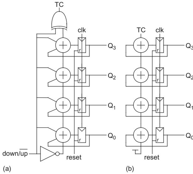
FIGURE 11.49 Synchronous counters
