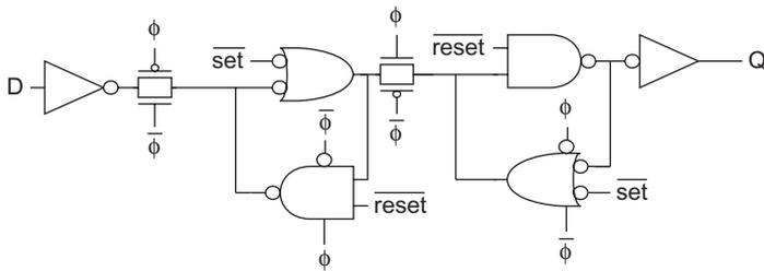
FIGURE 10.25 Flip-flop with asynchronous set and reset
