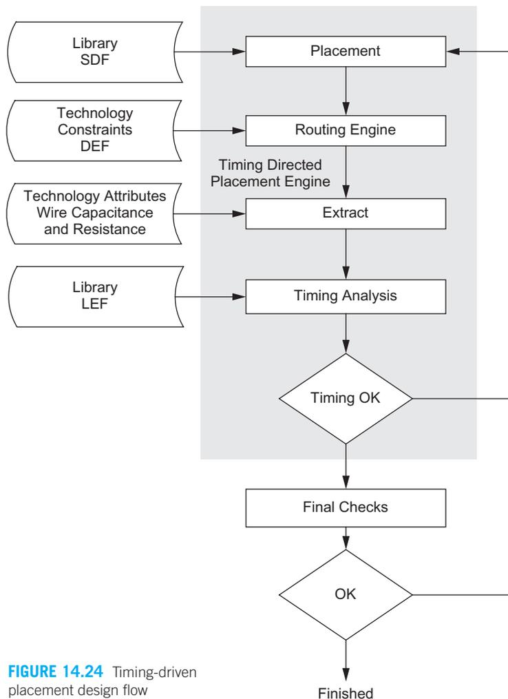
**FIGURE 14.24** Timing-driven placement design flow
