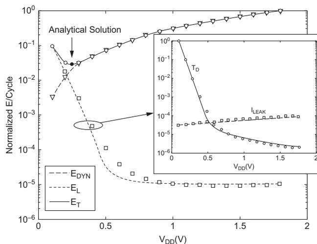
**FIGURE 5.26** Minimum energy point (Reprinted from [Calhoun05]. © 2005 IEEE.)
