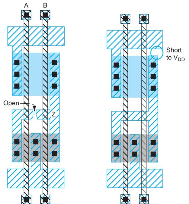
FIGURE 15.14 A defect that causes static  $I_{DD}$  current
