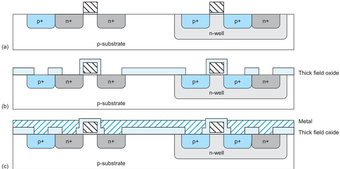
**FIGURE 1.38** Cross-sections while manufacturing p-diffusion, contacts, and metal
