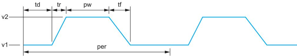
FIGURE 8.3 Pulse waveform
