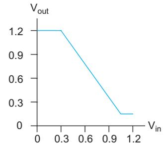
FIGURE 2.34 Transfer characteristics
