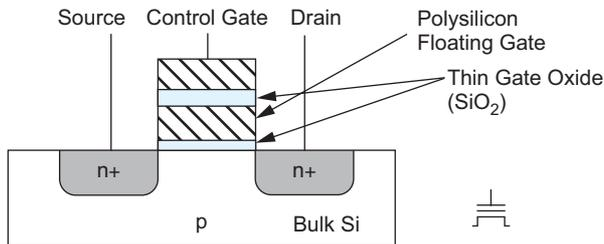
FIGURE 12.57 Cross-section of floating gate nMOS transistor
