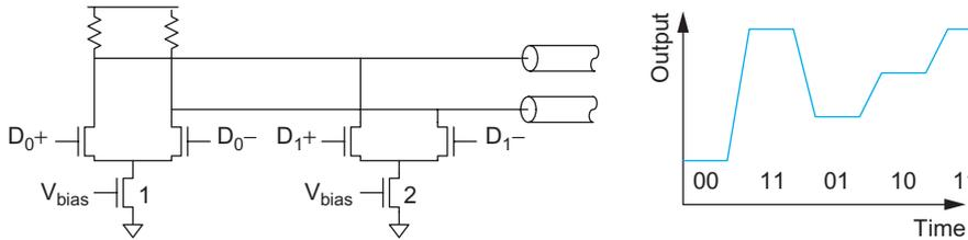
FIGURE 13.68 Multilevel transmitter
