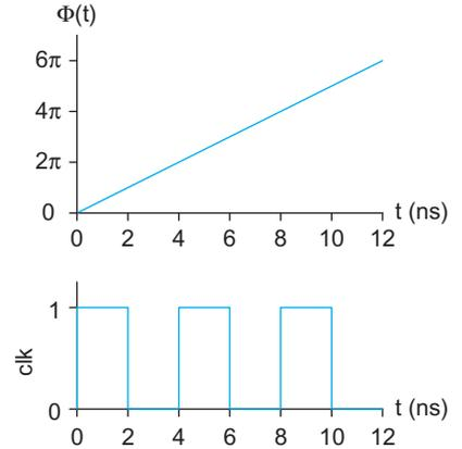
FIGURE 13.33 250 MHz clock phase and waveform
