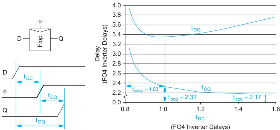
FIGURE 10.35 Flip-flop delay vs. data arrival time
