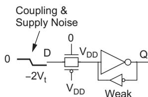
FIGURE 9.60 Noise on diffusion input of latch
