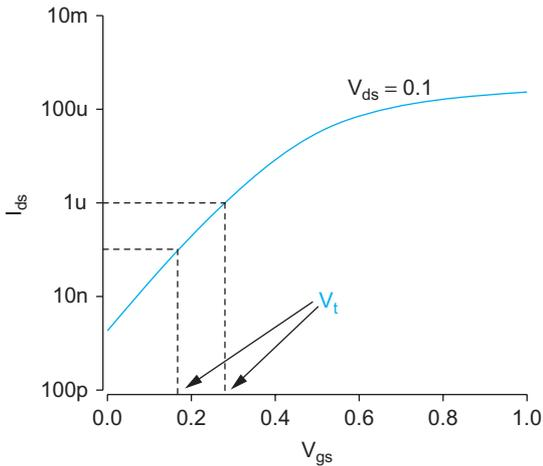
FIGURE 8.19 Constant current threshold voltage extraction method
