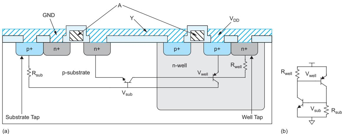
FIGURE 7.12 Origin and model of CMOS latchup
