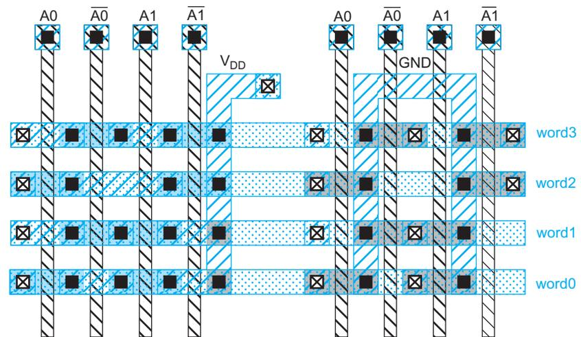
FIGURE 12.55 Row decoder layout on tight pitch
