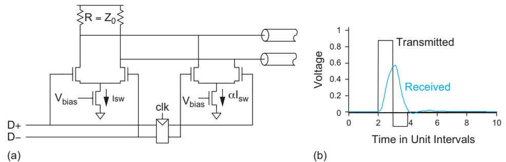
**FIGURE 13.66** De-emphasizing transmitter (a) circuit, (b) de-emphasized pulses
