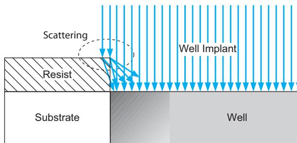
**FIGURE 3.6** Well-edge proximity effect, in which dopants scattering off photoresist increase the doping level near the edge of a well
