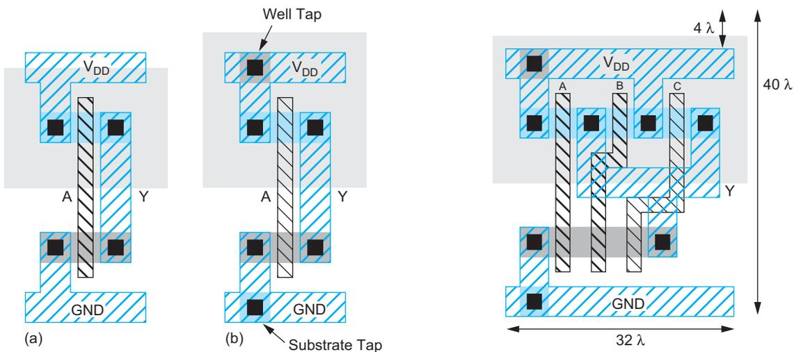
FIGURE 1.41 Inverter cell layout
