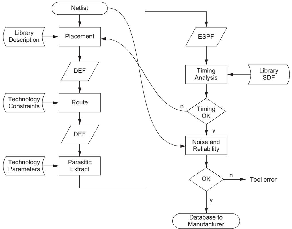
FIGURE 14.22 Standard cell place and route design flow
