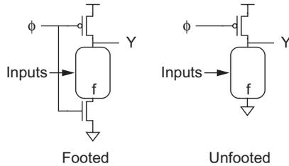
FIGURE 9.24 Generalized footed and unfooted dynamic gates
