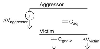
**FIGURE 6.17** Coupling to floating victim
