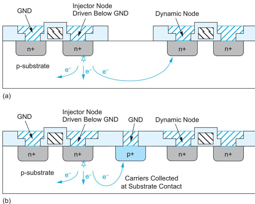
FIGURE 9.58 Minority carrier injection and collection
