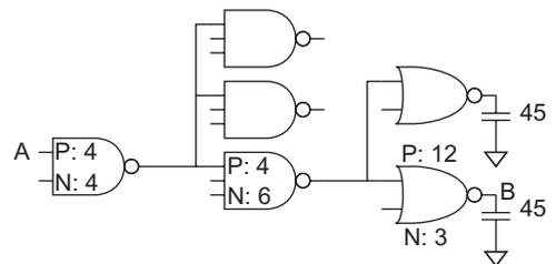
FIGURE 4.32 Example path annotated with transistor sizes
