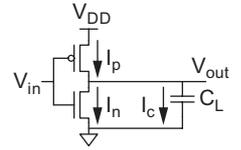
FIGURE 5.4 CMOS inverter
