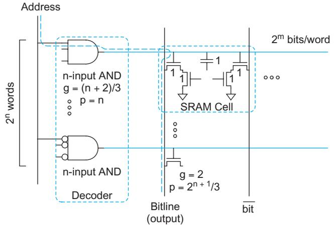
FIGURE 12.40 Critical path for read of small SRAM
