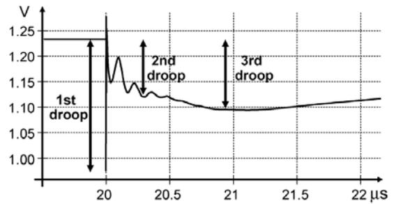
**FIGURE 13.13** Pentium 4 simulated voltage droops (© 2006 IEEE.)
