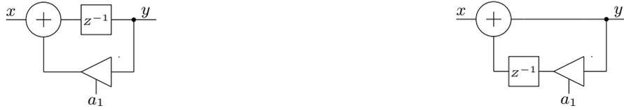
(a) Structure of a typical first order IIR filter.
