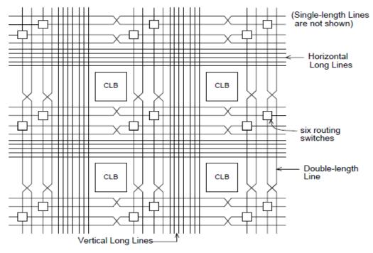
Fig 2.10 double length line and long lines
