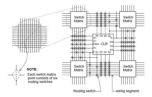
Fig 2.9 Routing structure
