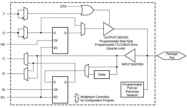
Fig 2.11 Input Output Block
