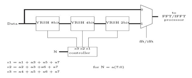
Here in this block all the VRSH blocks are controlled hard left shifters with a control input s. If s is equal to 1 then right shift take place otherwise passes as it is .For these case hardware minimization can be achieved as both the operation are not taking place at the same time .Several proposed designs [18] are available for implementing FFT /IFFT processors.
